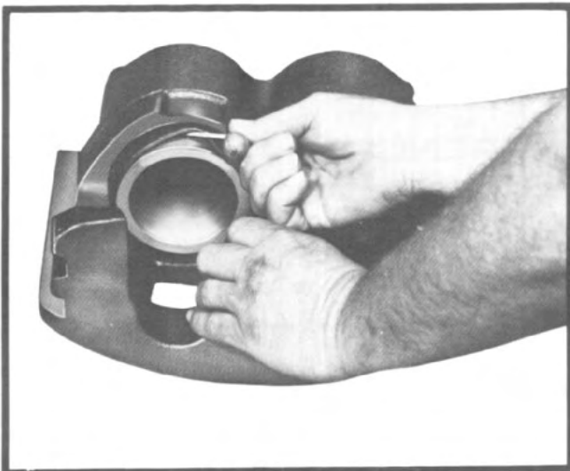
Fig. 32—Working boot around closed end of piston.
