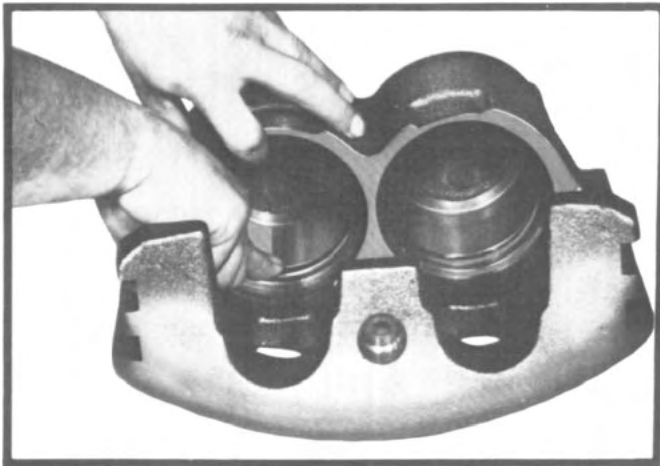
Fig. 31 — Installing piston seal in caliper groove.
