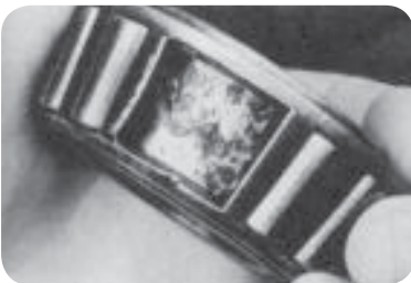
Spalling begins as small fractures under the bearing's surface. (fig. 5)
