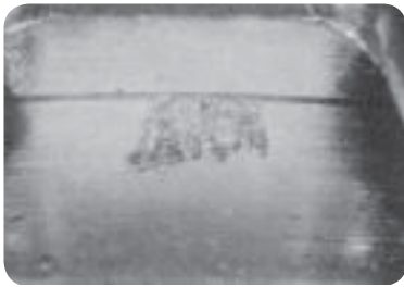
Electric currents passing through a bearing cause arcing and burning. (fig. 7)
