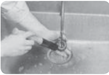
Rinse the bearing in clean solvent. (fig. 7)
