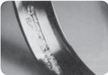
Friction caused by misalignment will discolor the roller path and rollers. (fig. 6)
