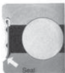
Seals prevent lubricants from leaking out of the bearing. (fig. 3)
