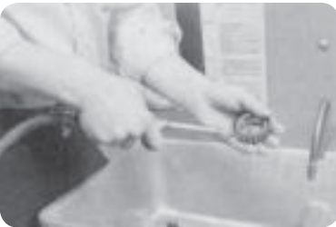
Compressed air may be used to dry the cleaned bearing. (fig. 8)
