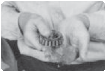
Grease the bearing. (fig. 9)
