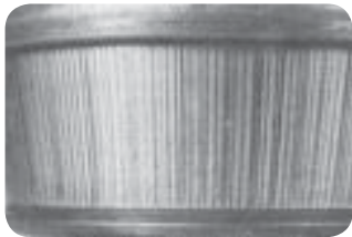
Electric current also causes grooves on the bearing. (fig. 8)
