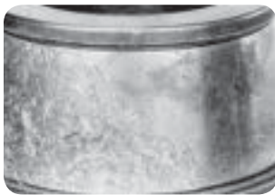
Inner race damage from misalignment. (fig. 5)
