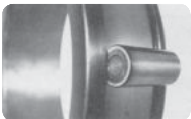
Seizing damage usually appears on the rollers. (fig. 9)
