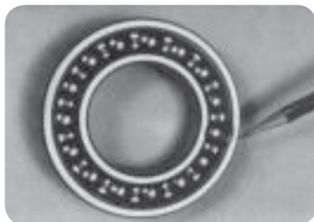
The maximum capacity bearing is a variation of the single row ball bearing. (fig. 7)
