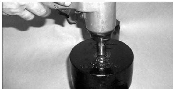
2. Remove all external seals from the steering gear, including the sector shaft dust boot, snap ring protective cover (if equipped), frame side protective disk and the input shaft dust boot.
