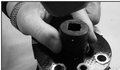
9. Clean the cover with a suitable solvent. If the cap you are working on has a grease fitting, remove the grease fitting and fill the hole with RTV compound. No further greasing is required.
