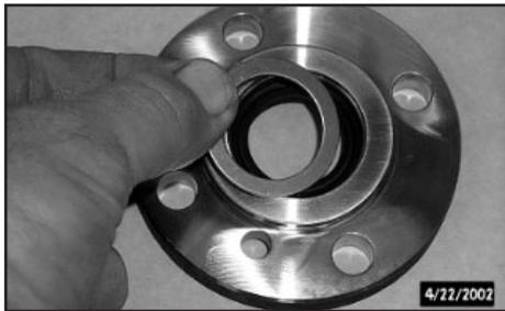
2. Install the protective washer (if equipped) into the bearing cap cover using an arbor press and suitable size seal driver. Install a new o-ring on the bearing cap cover.
