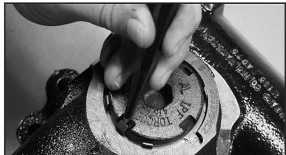
**IMPORTANT:** Do Not bend the aligning tabs out of the pitman arm.
