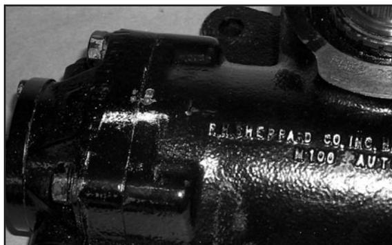
4. Remove the sector shaft cover using the appropriate tools for the steering gear you are working on. There are three methods of attachment for the sector shaft cover. Snap ring design, bolt on or clip style as shown.
