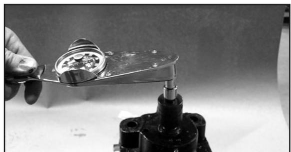
15. Install the locking nut over the shaft retaining nut. Using a spanner wrench tighten the locking nut until two tangs align with the oil flow holes of the bearing cap. Bend the locking tabs into the holes to secure the locking nut.
