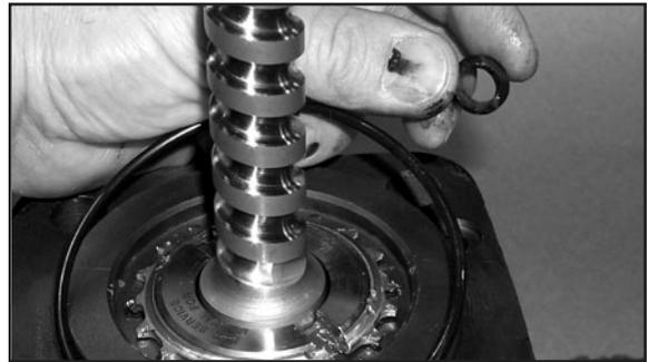
18. Install the plunger into the bearing cap. Reassemble the steering gear following the procedures in the re-assembly portion of this manual.
