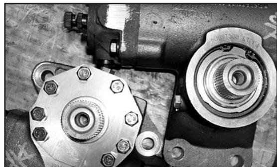
5. Clean the shaft and remove the sector shaft cover. It may be necessary to crank the engine to force the cover out of the housing
