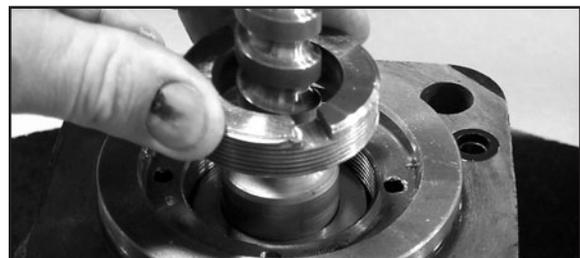
**IMPORTANT:** Do not remove the rotary valve seals!
