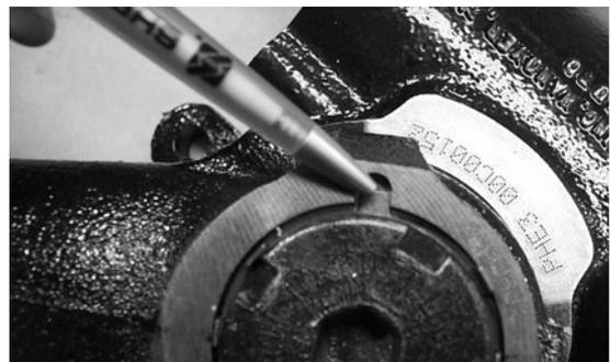
**IMPORTANT:** Take note of the torque value on the face of the retainer. Always torque the retainer to the specified value.
