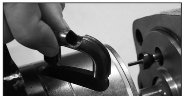
11. Replace the O-ring on the ball guide retainer and install the ball guide retainer over the ball return tubes.
