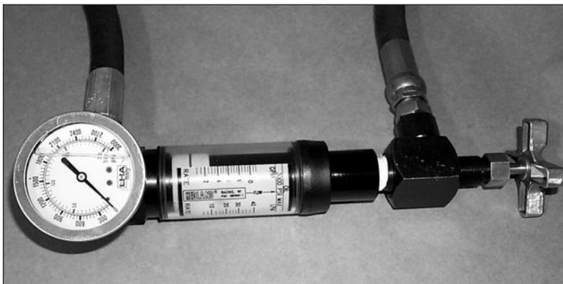
This tester is a self contained, direct reading device to check system flow, pressure or both at the same time. It can detect worn components, check flow and pressure control settings or monitor overall system performance.
