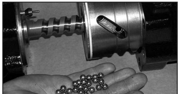
15. Remove the bearing cap and shaft assembly from the piston. Place the bearing cap and shaft assembly on a clean work surface. If equipped with manual plungers, remove the plunger at this time. Follow the Auto Plunger Repair procedure in the Common Procedures section for Auto Plunger equipped steering gears.
