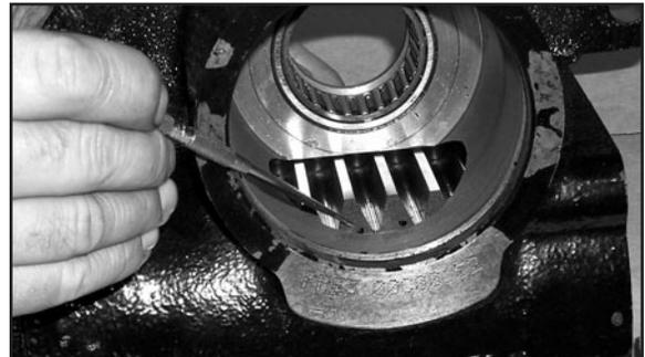
14. Align the marks on the bearing cap with the marks on the housing. Install the four attaching bolts in the bearing cap assembly and torque to specifications.
