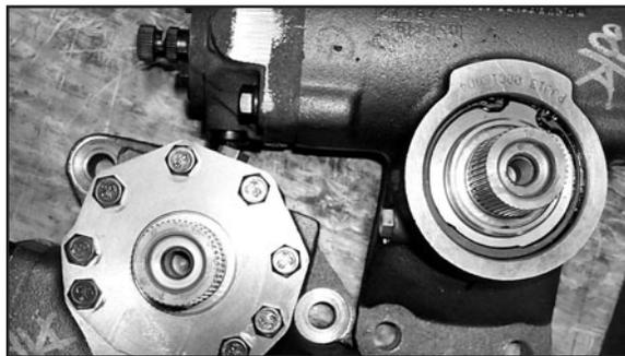
17. Install the sector shaft cover onto the steering gear. It may be necessary to drive the cover on with a dead blow hammer. Attach the cover using the appropriate tools for the steering gear you are working on.
