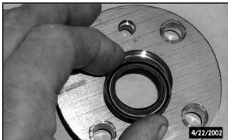
3. Press the salt seal into the cover until it is flush with the face of the cover. There is a choice of two salt seals for the M-series gear. Select the proper salt seal for your cover and press it into the cover until it is flush with face of the cover.
