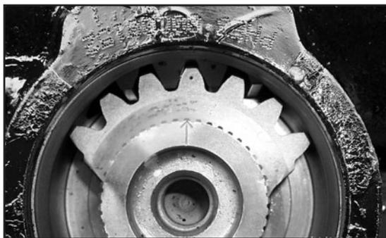
10. Install the sector shaft cover onto the steering gear. Insure that the cover is properly seated when installing. Snap ring covers must be flush or below the snap ring groove when properly installed.
