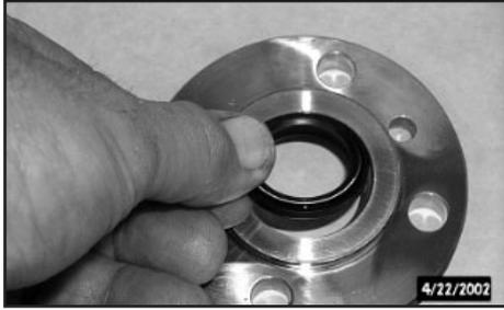
1. Place the cover face down on a clean work surface. Coat the outside diameter of the seal with clean chassis lube. Install the oil seal in the cover using a suitable size seal driver and an arbor press. Make sure the lip of the seal faces up when installing the seal.
