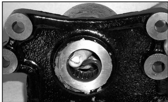
9. Install the sector shaft into the housing taking care to align the timing mark on the sector with the timing marks on the piston. It may be necessary to tap on the sector shaft to properly seat it into the housing.
