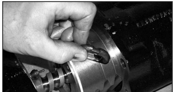
14. Carefully turn the shaft to remove the re-circulating balls from the piston. All M-Series steering gears will have 24 balls. Verify that all balls are removed before removing the valve shaft from the piston.
