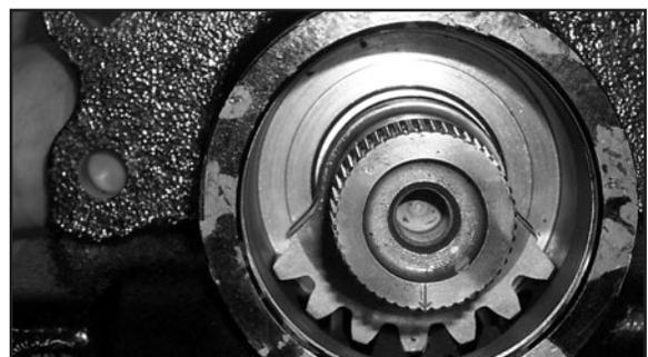
16. Install a new sector shaft oil seal in the sector shaft cover. When properly fitted the seal will ride between the roller bearing and cover. The black lip of the seal must face the bearing.
