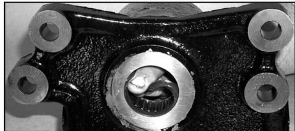
**IMPORTANT:** The sector shaft seal is a two piece seal. It will necessary to bend the seal for installation. Once the seal is installed you may have to work the seal into place with your fingers or a blunt seal pick to properly seat the seal. Press only on the body of the seal.
