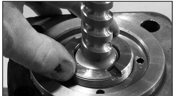
**NOTE:** Valve pre-load can be measured by turning the input shaft with an inch pound torque wrench. When properly set the radial drag will not exceed 25 inch pounds.
