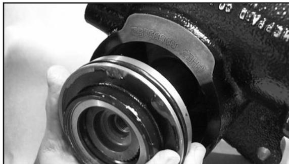
**IMPORTANT:** Coat the seal area of the sector shaft with grease to prevent seal damage at installation.
