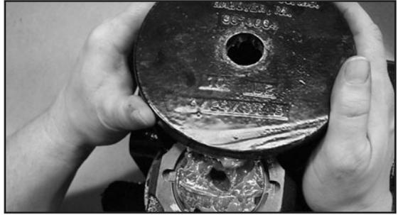
**NOTE:** It will be necessary to remove the sector shaft cover bolts to slide the puller over the arm if the gear you are working on has a bolt on cover.
