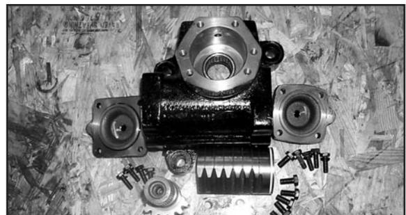
Sheppard Power Steering gears have no external adjustments for sector shaft or valve shaft pre-load. Make sure all linkages and system components are within vehicle manufacturers specs.
