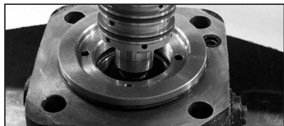
6. Remove the outer thrust assembly from the bearing cap bore. Note the order of assembly for reassembly.
