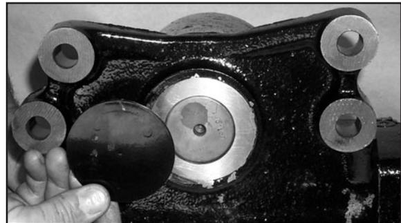
22. Install the snap ring protective cover in the sector shaft cover bore over the snap-ring by lightly tapping on the outside diameter. Install the slide on V-boot over the sector shaft. Install the rubber boot on the input shaft.
