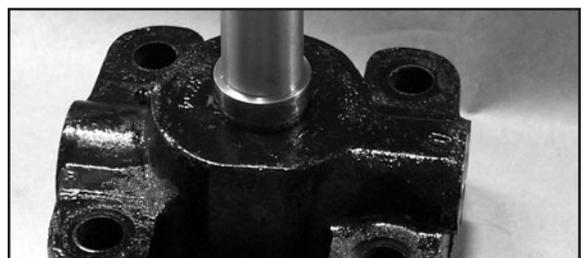
11. Tape the input shaft splines to prevent seal damage. Place the outer thrust assembly on the rotary valve. The thrust bearing will go toward the valve, the thrust washer will ride on the bearing cap surface.
