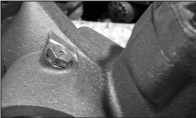
16. Using the allen wrench open the bleeder screw until non-aerated fluid flows from the bleed screw.
