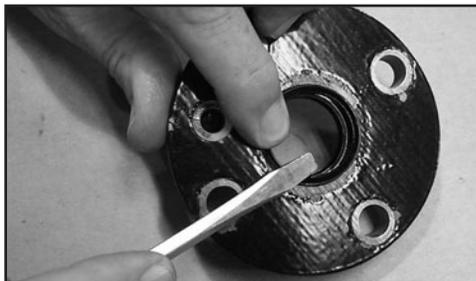
7. Place the bearing cap cover on a clean work surface. Pry the salt seal out of the bearing cap cover.
