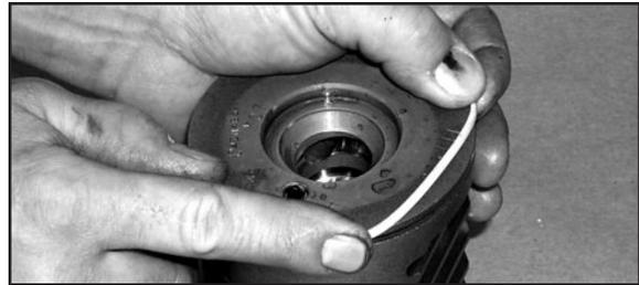
2. Install a new sector shaft oil seal in the housing. When properly fitted the seal will ride between the roller bearing and housing lip. The black lip of the seal must face the bearing.
