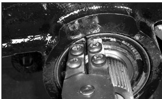
12. Using an appropriate size seal driver, install the excluder seal in the cover. Apply a coat of clean chassis lube in the lip of the seal before installing. Apply a bead of grease over the excluder seal and slide the rubber boot over the sector shaft.
