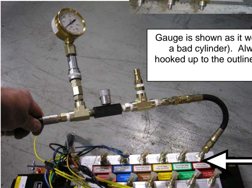
Gauge is shown as it would be installed on a pump (checking a bad cylinder). Always install the gauge on the hoses hooked up to the outlined color side of the decal, not the solid color side.
