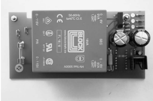
Illustration: Power-pack board, front and back
