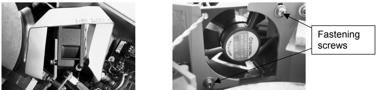
Illustration: Fan underneath the ribbon cable, fan fastening screws
