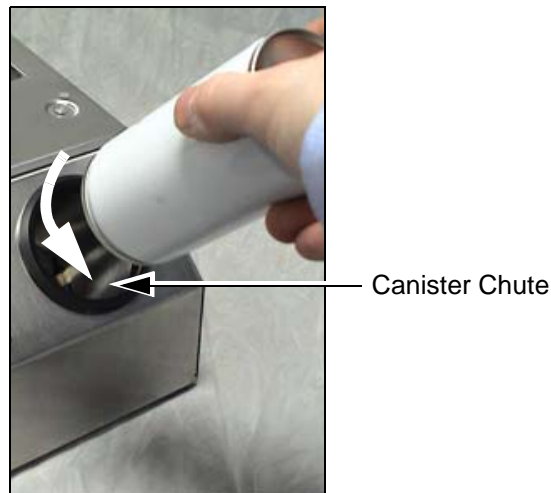
Figure 4-11: Removal of Empty Ink Canister
