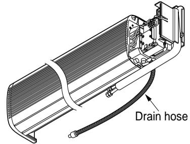
**2. Insert the piping, drain hose and the connecting cable into the piping hole.**
