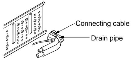
**3. Insert the connecting cable into the indoor unit.**
