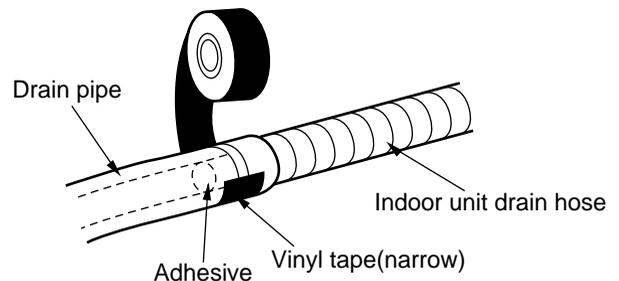
**6. Wrap the insulation material around the connecting portion.**
