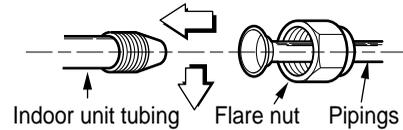
■ Tighten the flare nut with a wrench.
