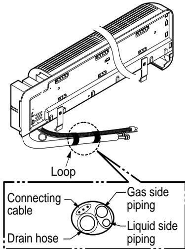
**NOTE:** If the drain hose is routed inside the room, insulate the hose with an insulation material\* so that dripping from "sweating"(condensation) will not damage furniture or floors.
