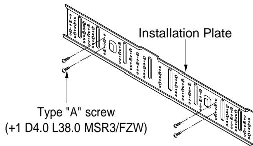
**2. Measure the wall and mark the centerline. It is also important to use caution concerning the location of the installation plate—routing of the wiring to power outlets is through the walls typically. Drilling the hole through the wall for piping connections must be done safely.**
