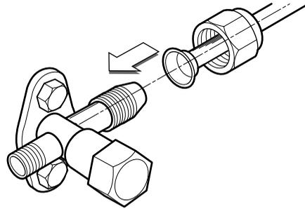
2. Finally, tighten the flare nut with torque wrench until the wrench clicks.
