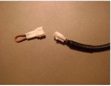
Plug in the OFT Moto-r Kill's <u>female</u> white OEM style connector to the harness coming in from sled (red /brown wires – yellow circle). Insert "test plug" into the remaining <u>male</u> Moto-r Kill harness connector. Leave OEM connector that goes to handlebar kill switch (green circle) disconnected and tucked in wiring cover. Insert any remaining wiring into wiring cover, and close up with zip ties.
