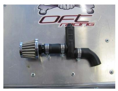
NOTE: Ensure hoses are attached exactly as shown above so inlet and outlet of valve is plumbed correctly.
