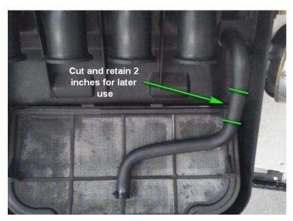
You will be left with approximately what you see below. Remove 3/4" from the end that attaches to the crankcase pipe fitting in the air box, then measure 3" around the OUTSIDE of the pipe radius. Cut the pipe, and retain this 90 for later attachment to the Jake valve.
