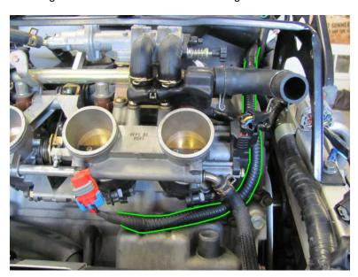
Install 90 degree bend breather tube of Jake valve to crankcase fitting and parallel to the throttle bodies using OEM squeeze clamp as shown:
