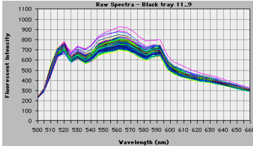
**Note** Signal heights vary depending on the well position, the specific ABI PRISM 7700 instrument being used, and the temperature of the test tray. Results obtained from using a blackboard do not take into account background signal from the sample block or real PCR samples.
