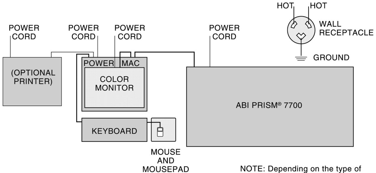
NOTE: Depending on the type of monitor used, its power cord MAY plug into the back of the PowerPC Macintosh.
