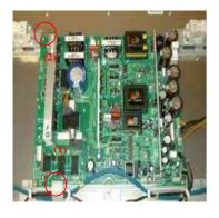
1.Unplug the signal transmitting connector for the PANEL BUS at the butto 2.Change the POWER BOARD by removing the 8pcs screws(M3X6) on each corner.
