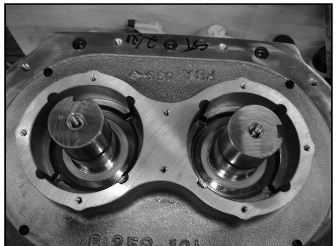
Figure 3B – Bearing Shims Installed
