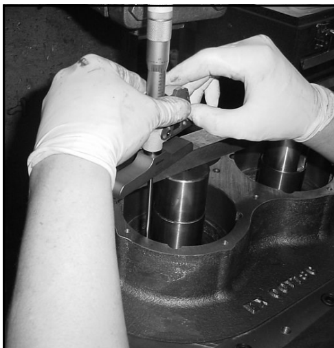
Figure 3A – Determining amount of Bearing Shims Needed
