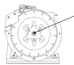
6. Remove the Philips screw, and spring in the centre of the disc. The disc assembly is now free floating in the hopper, remove the assembly by pulling on the agitator and lift it from the motor shaft.
