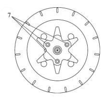
7. Remove the 3 hex key screws, and disassemble the whole disc to make the new requested combination.
