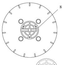
8. Take requested pinwheel, shelf-wheel and agitator, and mount the 3 screws back in position.
