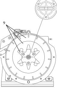
9. Put the disc assembly back on the hopper. The disc only fits 2 ways into the driver pin.
