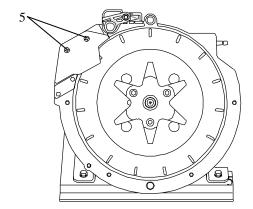
5. Remove the 2 Philips screws, which holds the coin deflector, and remove the coin deflector.
