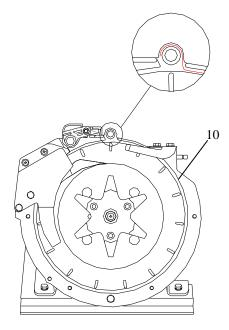
Place the spring liner in position around the disc, make sure the end of the spring liner fits correct in the upper part on the wheelhousing.
