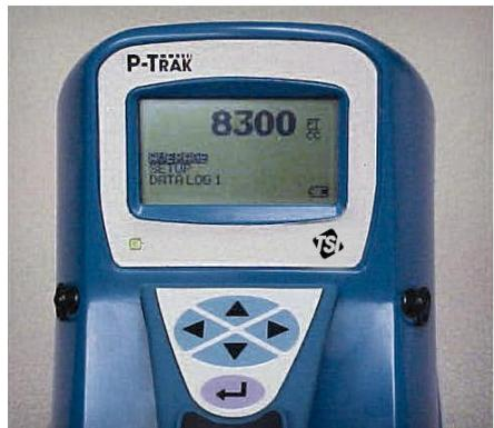
**Figure 3-1: P-Trak Particle Counter Keypad and Display**
