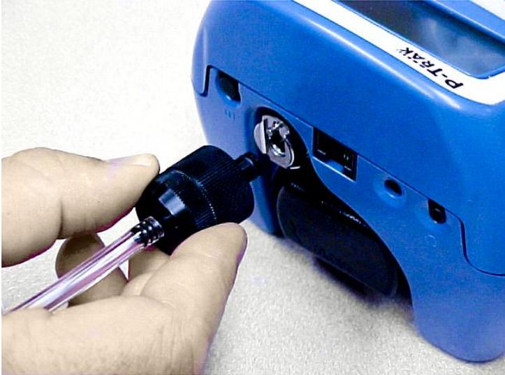
**Figure 2-7: Insert Inlet Screen Assembly into Fitting**
