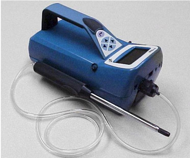
**Figure 2-8: Slide Telescoping Probe onto Instrument Case**
