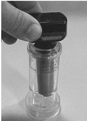
Figure 2-5: Insert Alcohol Cartridge into Fill Capsule
