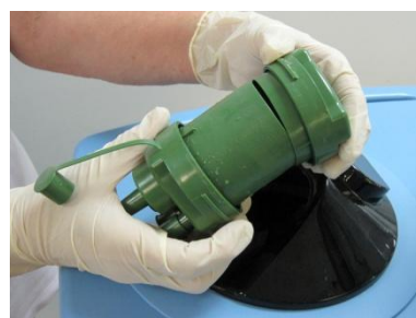
Figure 14 – Used Manifold Removal
