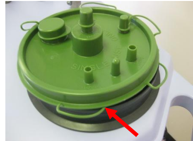
Figure 18 – Port Cap Under Lid
