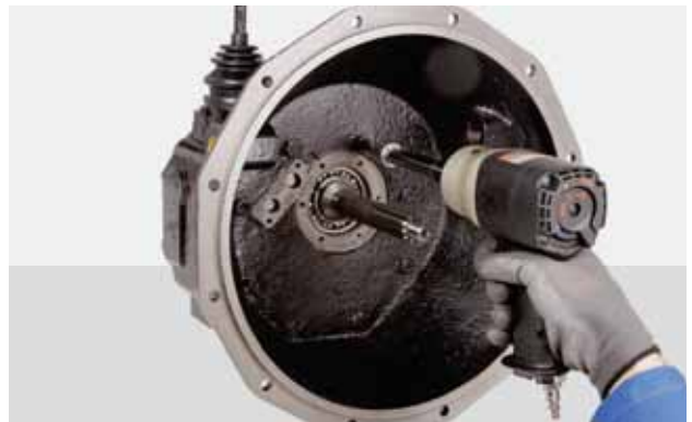
FIGURE 17: Loosen and remove the clutch housing screws.
