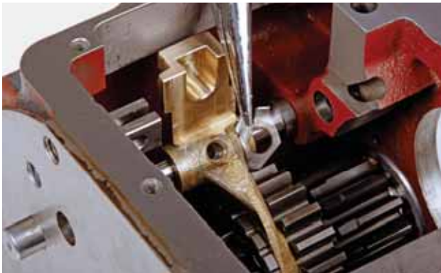
FIGURE 77: Install the position stop in its seat.
