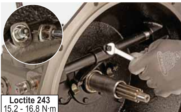
FIGURE 120: Assemble washer and nut and tighten.
