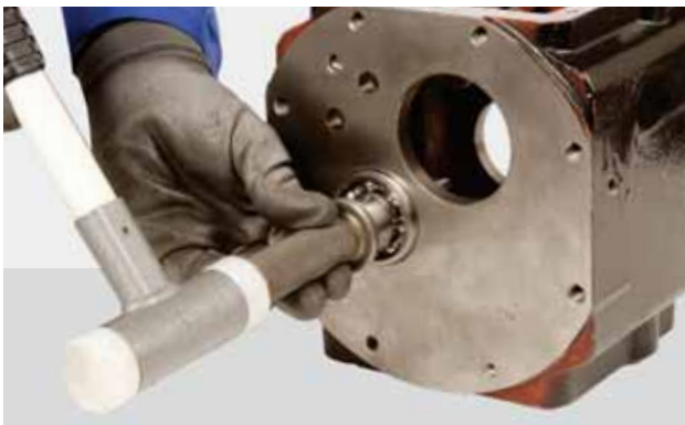
FIGURE 57: Remove the bearing.
