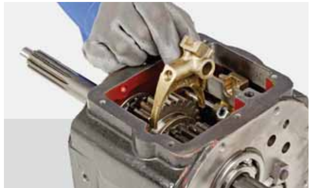
FIGURE 93: Engage the fork in the coupling.
