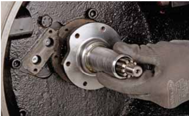
FIGURE 15: Remove the sleeve.
