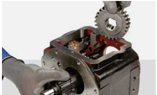
FIGURE 87: Fit the 2nd gear onto the input shaft.
