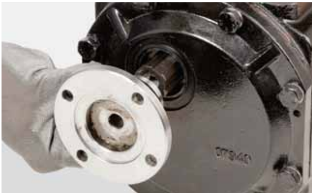
FIGURE 27: Remove the flange.
