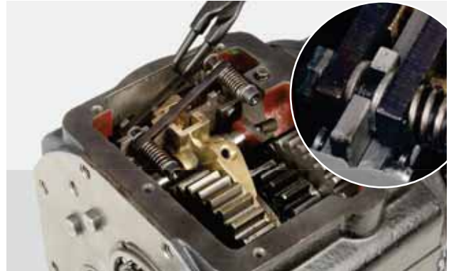
FIGURE 103: Fit the gear selector yoke in position.
