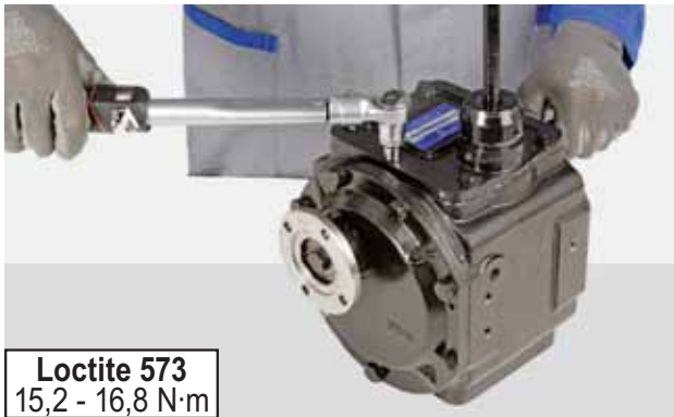
FIGURE 106: Apply and tighten the screws securing the gear selector cover, with their respective washers. Tighten to a torque of 15,2 - 16,8 N·m.
