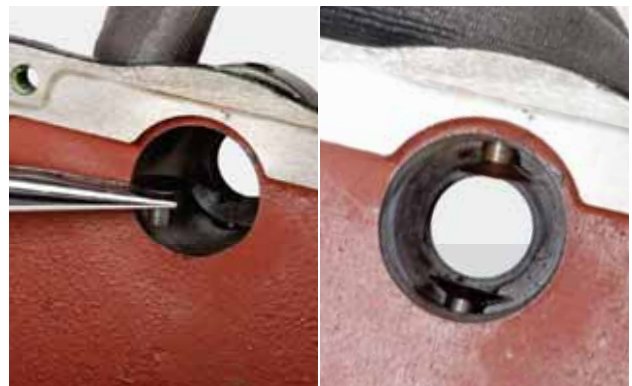
FIGURE 104: Install the lever adjustment pins.
