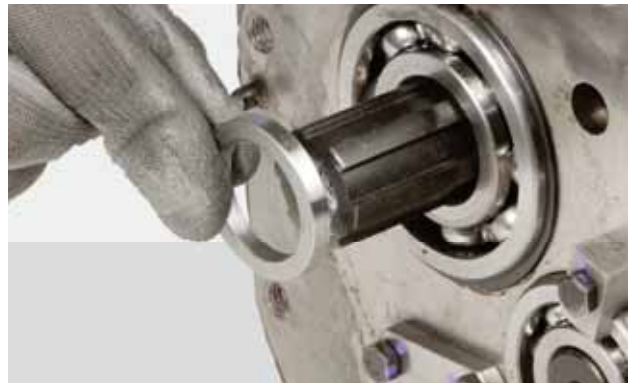
FIGURE 30: Remove the spacer.
