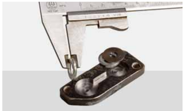
FIGURE 12: Measure and write down shim quantity and position. Do not switch shim locations.
