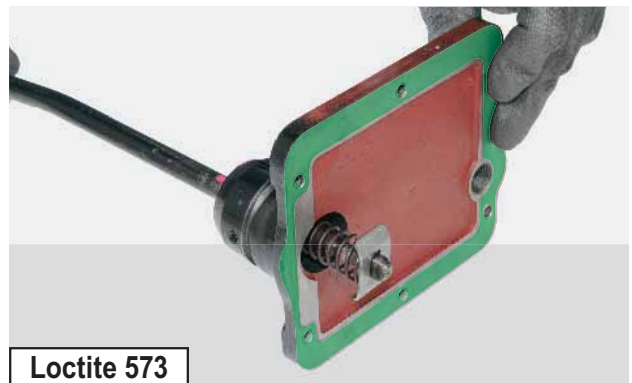
FIGURE 105: Apply LOCTITE 573 to the machined surfaces, and fit the gear selector cover on the housing.
