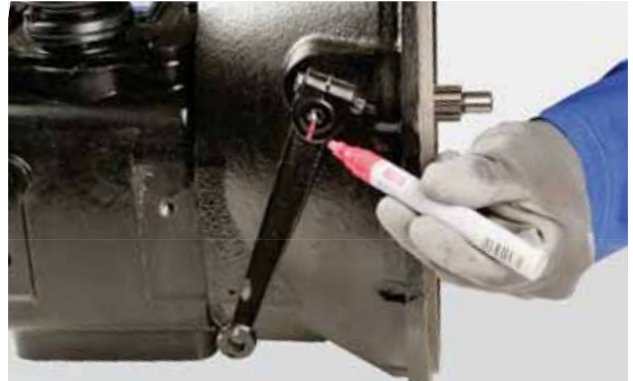
FIGURE 4: Mark the positions of levers in relation to the thrust lever.
