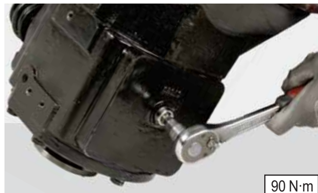
FIGURE 123: Install the plug and tighten to 90 N·m.
