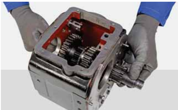
FIGURE 55: Remove the secondary shaft.
