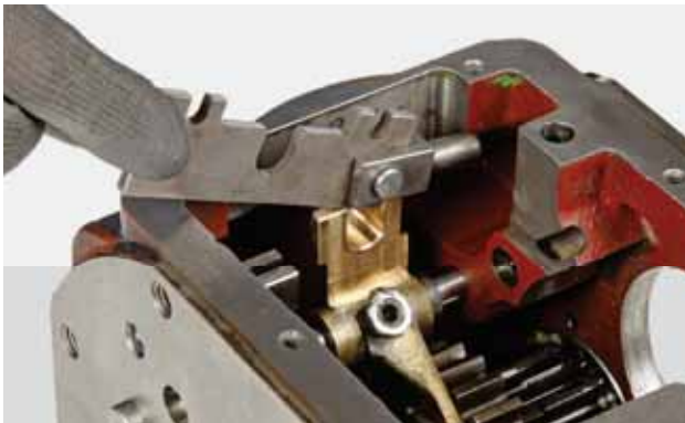
FIGURE 45: Remove the gear selector bar.
