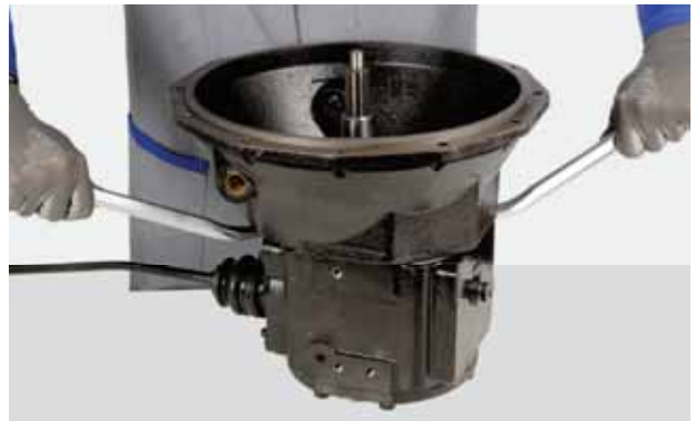
FIGURE 18: Remove the clutch housing.
