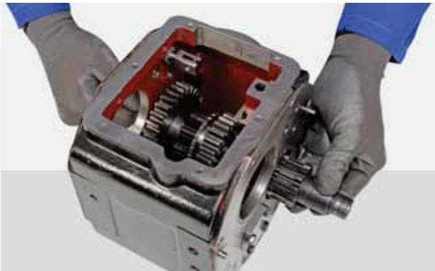
FIGURE 70: Install the secondary shaft.
