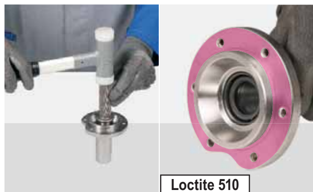
FIGURE 111: Using the special tool T3 (see drawing T3 p. 38), install the seal ring into the sleeve.
