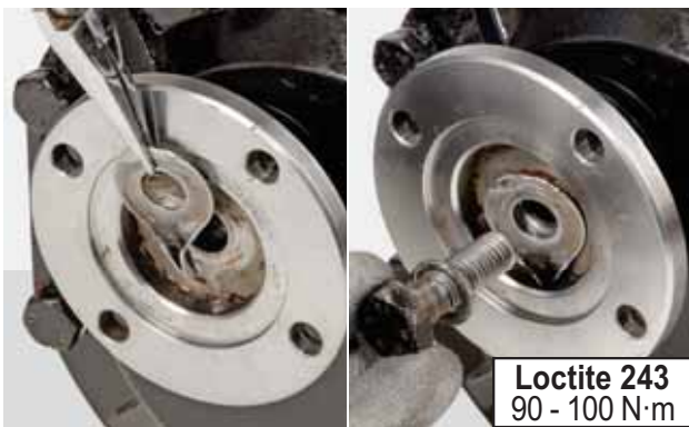
FIGURE 101: Apply the T2 tool (see drawing T2 p. 37) onto the flange. Secure the wrench and tighten the screw using a torque wrench, up to a minimum required torque setting of 90 - 100 N·m.
