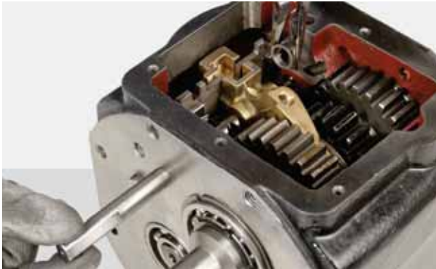
FIGURE 94: Insert the control rod and install the spacer.
