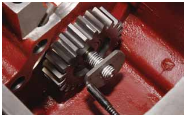
FIGURE 59: Write down the baffle plate position and remove.
