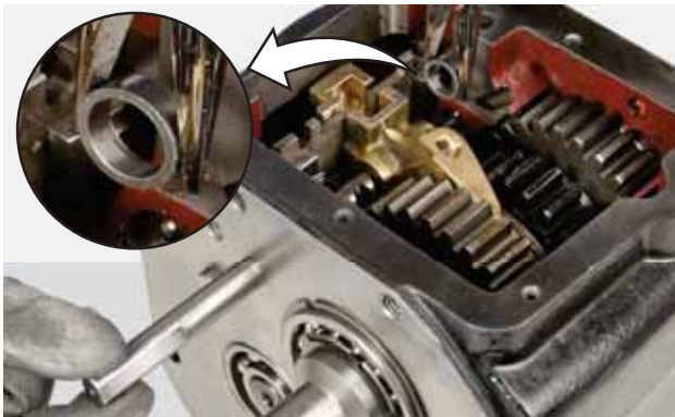
FIGURE 33: Partially extract the control rod and remove the spacer. Then completely remove the control rod.
