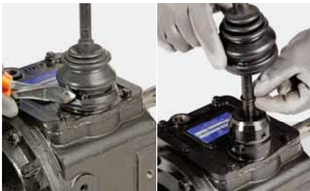
FIGURE 19: Cut the retainer clip and remove the protective boot and o-ring.
