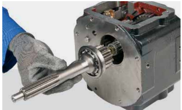
FIGURE 36: Remove the input shaft.
