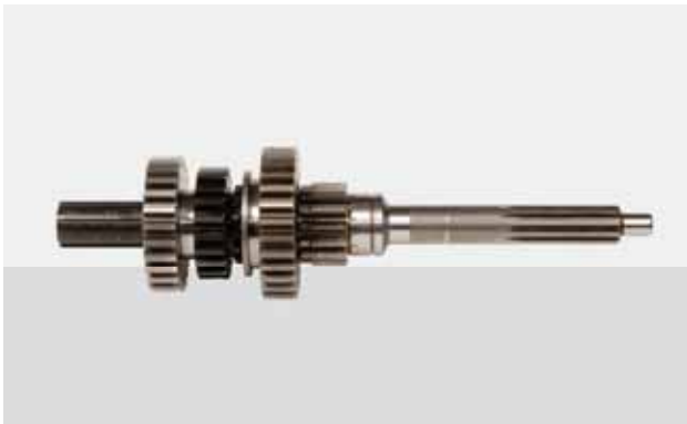
FIGURE 84: 1st - reverse gear shaft composition.
