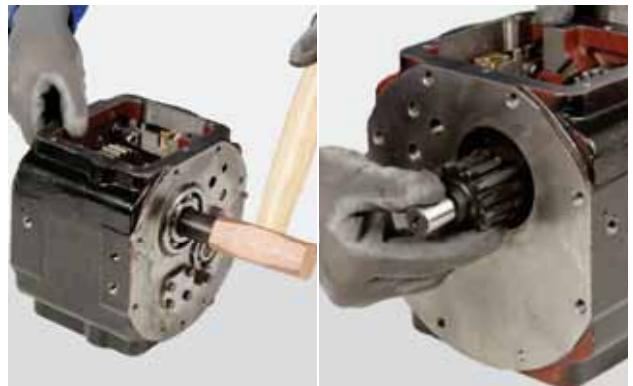
FIGURE 41: Gently tap to remove the input shaft.
