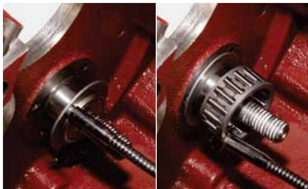
FIGURE 66: Install the spacer. Lubricate and fit the roller bearing.
