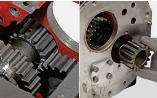
FIGURE 71: Install the reverse gear ratio gear.
