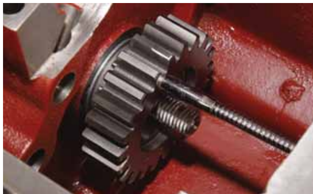
FIGURE 60: Remove the idler gear.
