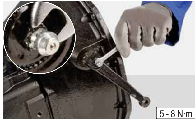
FIGURE 122: Install the grease zerk. Torque wrench setting: 5 - 8 N·m.
