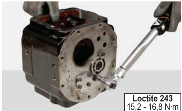
FIGURE 74: Install the mechanical endstops. Coat the screws with Loctite 243 and tighten to 15,2 - 16,8 N·m.
