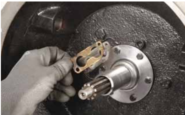
FIGURE 114: Install the paper gasket using the marking made previously as reference.
