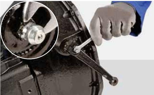
FIGURE 3: Only if necessary, remove the grease zerk.
