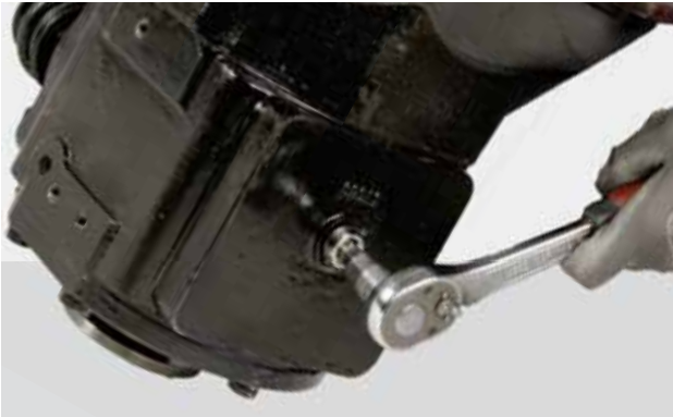
FIGURE 1: Remove the oil drain plug and drain oil.
