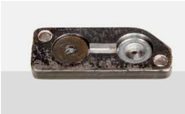
FIGURE 113: Restore the shims in the same position and quantity previously marked.
