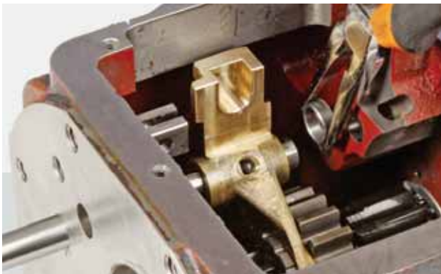
FIGURE 50: Partially extract the control rod and remove the spacer, then completely remove the control rod.
