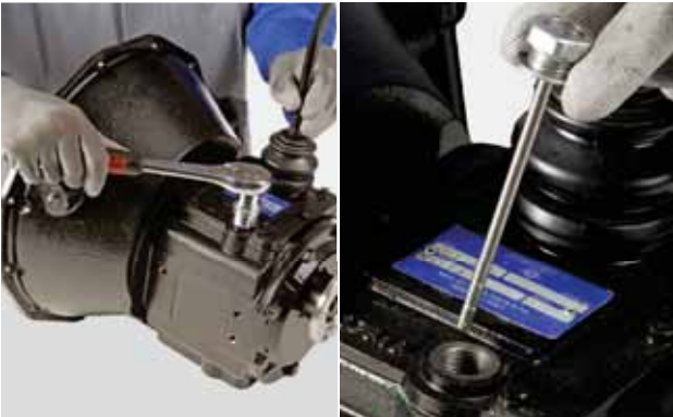
FIGURE 2: Remove the dipstick.
