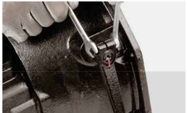
FIGURE 5: Loosen and remove nut, screw, and washer.
