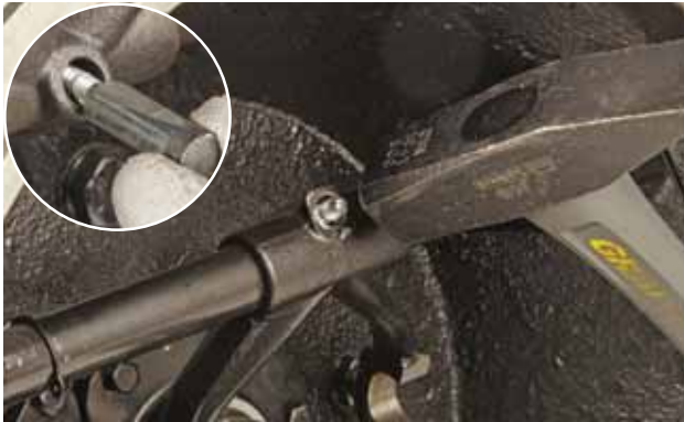
FIGURE 7: Using a copper hammer, gently tap and remove the conical pin of the yoke.
