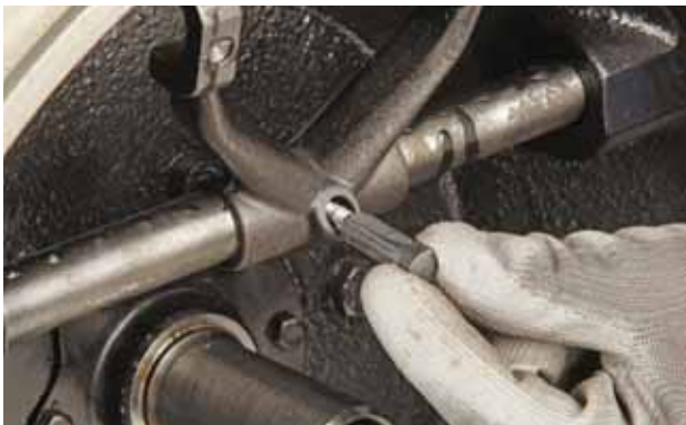
FIGURE 119: Align the pressure plate yoke with the hole and assemble the conical pin.
