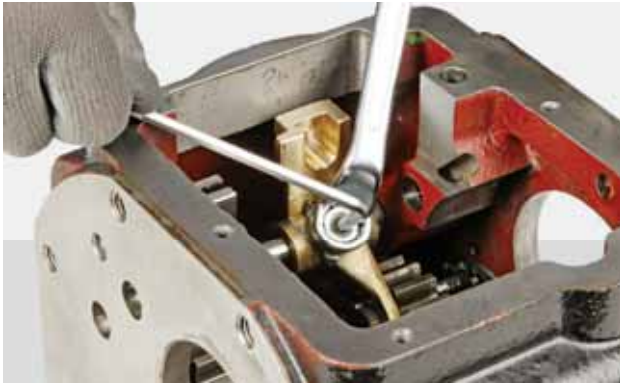
FIGURE 49: Loosen the counternut and remove the screw.
