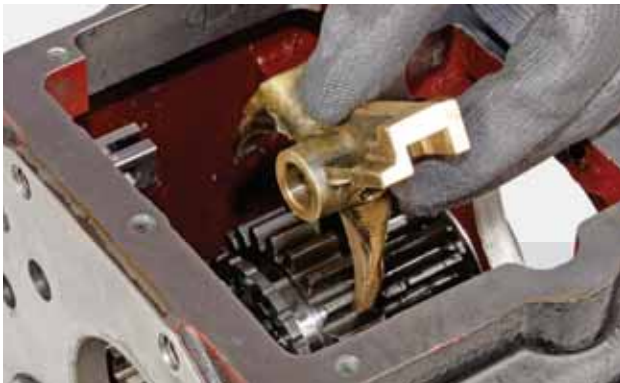
FIGURE 51: Write down the fork position and remove.
