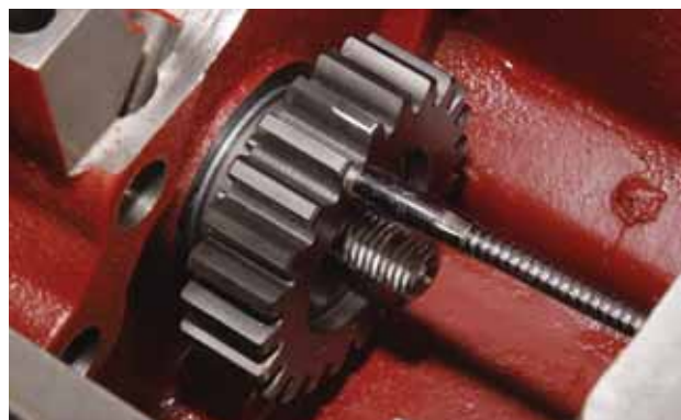
FIGURE 67: Install the idler gear.
