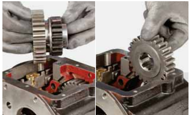
FIGURE 42: Remove 2nd and 3rd gear and sliding sleeve.
