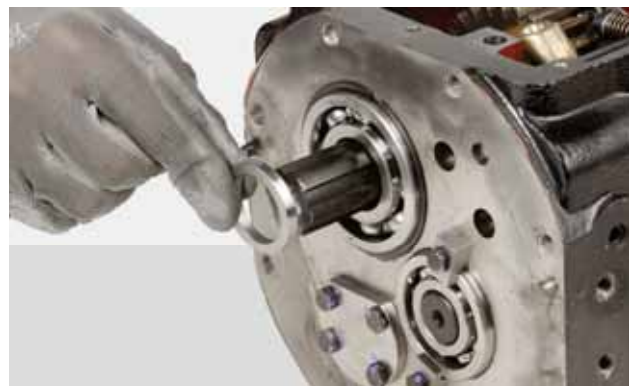
FIGURE 98: Install the spacer onto the output shaft.
