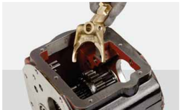
FIGURE 75: Engage the fork in the coupling.
