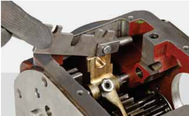
FIGURE 82: Insert the gear selector bar in the housing.
