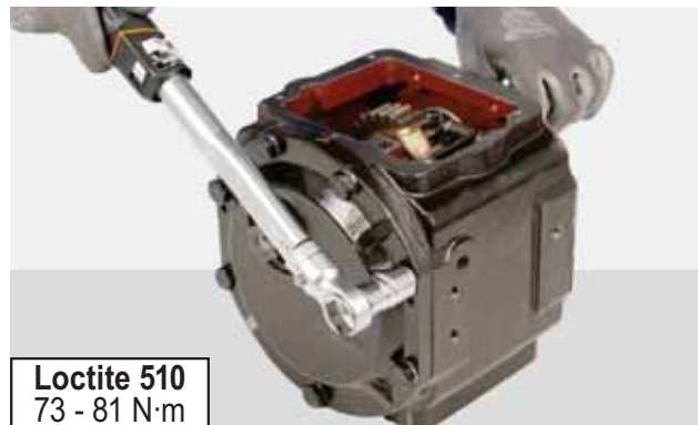
FIGURE 99: Fit the cover onto the casing and align the pins.
