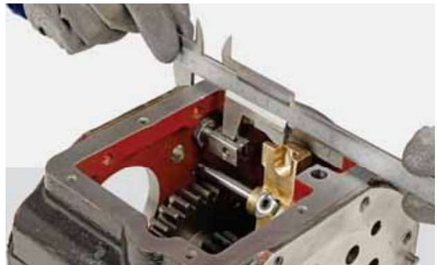
FIGURE 81: Only if removed, restore the position of the support according to the measurement previously taken. Coat threads with Loctite 243 and tighten the nut to a torque of 50 - 55 N·m.
