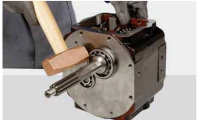
FIGURE 91: Using a copper hammer, insert the bearing in position.
