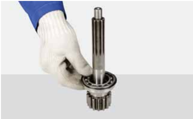
FIGURE 89: Heat the bearing up to 212°F [100°C] and install it onto the input shaft.
