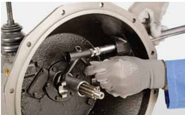
FIGURE 9: Remove the pressure plate fork and stud.
