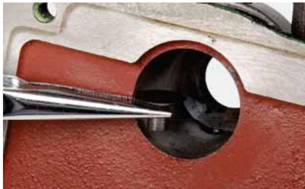
FIGURE 22: Remove the lever adjustment pins.
