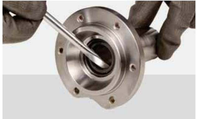
FIGURE 16: Using an extractor, remove the seal ring.
