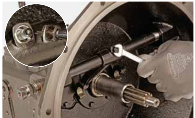
FIGURE 6: Loosen and remove the nut.
