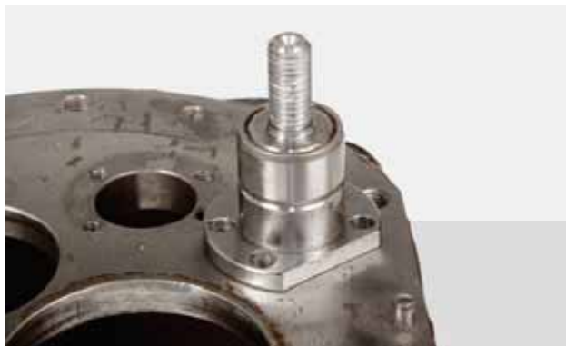
FIGURE 64: Install the complete idler gear support.
