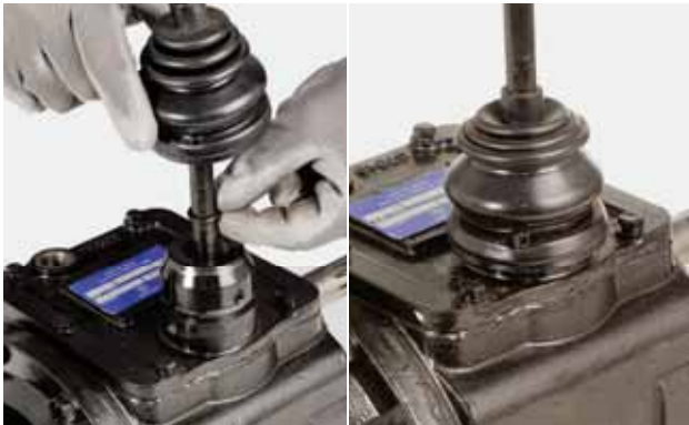
FIGURE 108: Install the protective boot and secure with clips.
