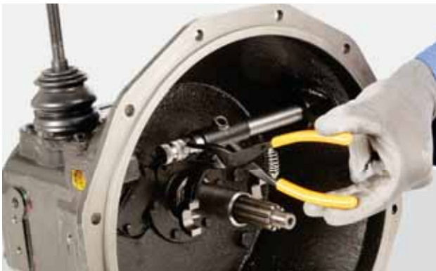
FIGURE 8: Remove the snap ring.
