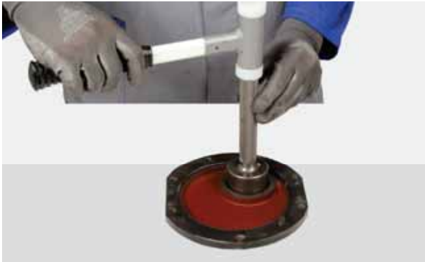
FIGURE 31: Use a driver to remove the seal ring.
