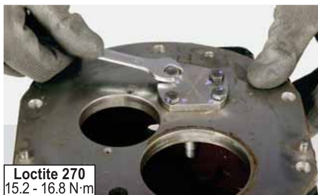
FIGURE 65: Spread the screws with Loctite 270 and tighten to a torque of 15.2 - 16.8 N·m.
