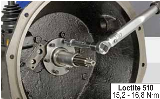
FIGURE 112: Coat the screw threads with Loctite 510 and tighten to a torque of 15,2 - 16,8 N·m.
