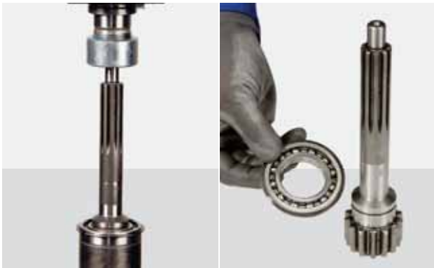
FIGURE 39: Position the input shaft under a press, and using a suitable drift, remove the ball bearing.
