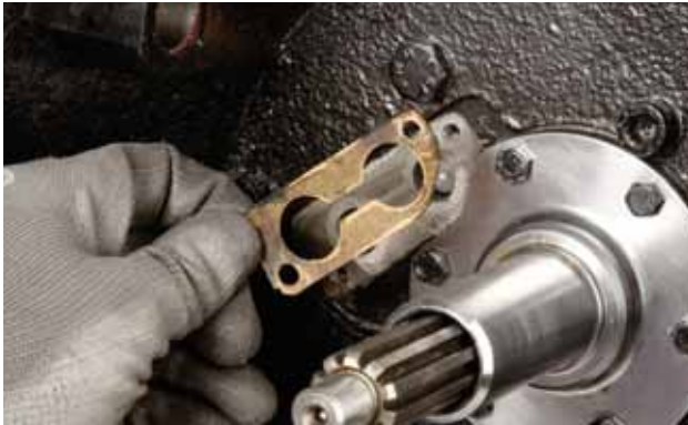
FIGURE 13: Remove the paper gasket.
