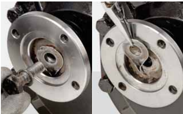
FIGURE 26: Remove the stop.
