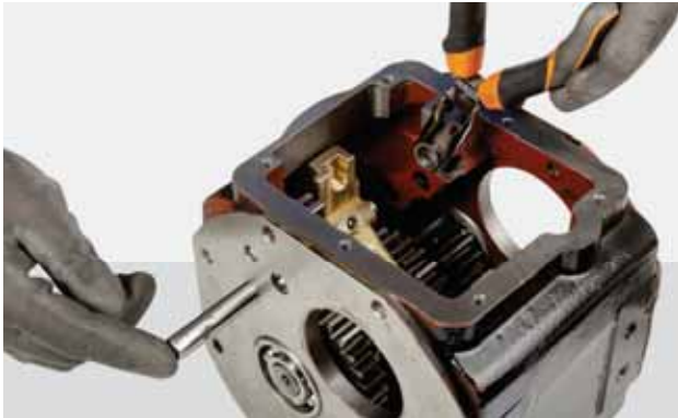
FIGURE 76: Insert the control rod and the spacer.
