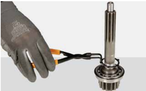
FIGURE 38: Remove the snap ring.
