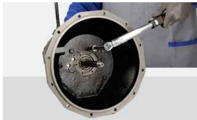
FIGURE 110: Coat the screw threads with Loctite 510 and tighten to the following torque specifications: M8: 35 - 40 N·m. M10: 70 - 75 N·m.
