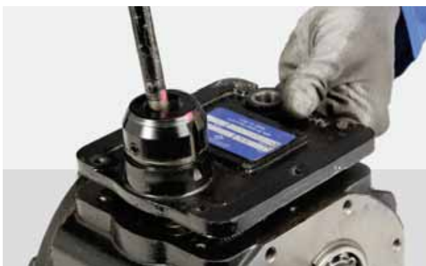
FIGURE 21: Remove the gear selector cover.
