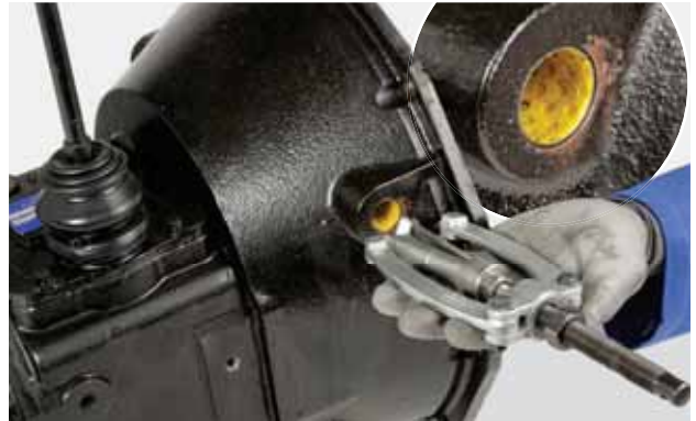
FIGURE 10: Using an extractor for inner parts remove the bushings.
