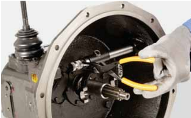
FIGURE 118: Install the snap ring. Carefully check snap ring is completely inserted.
