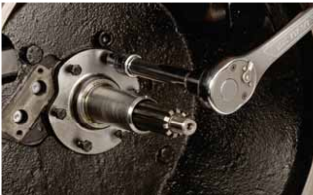
FIGURE 14: Remove the capscrews and washers.
