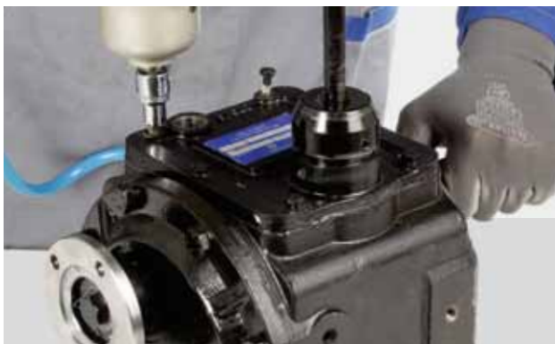
FIGURE 20: Remove the screws securing the control lever cover, together with washers.
