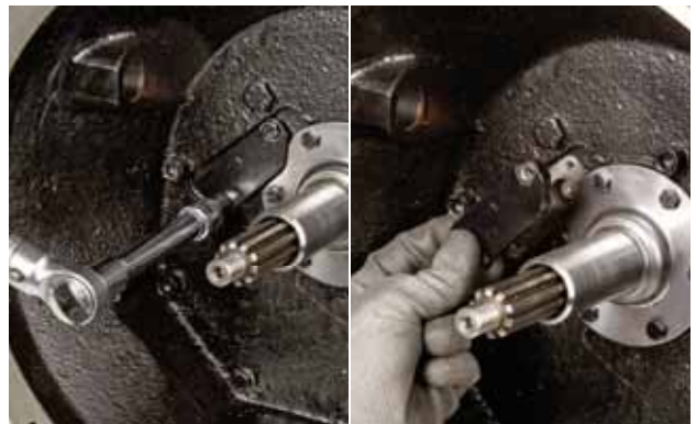
FIGURE 11: Remove the shift rail cover.
