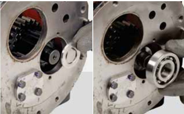
FIGURE 72: Install the spacer and bearing.
