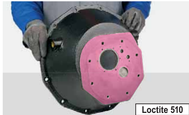
FIGURE 109: Coat the surface of the main body with Loctite 510 and install the support.
