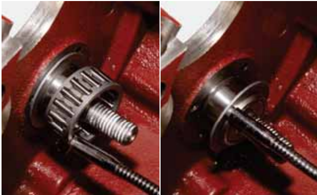
FIGURE 61: Remove the roller cage bearing and washer.
