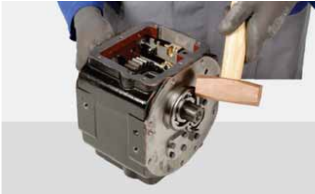
FIGURE 88: Using a copper hammer, insert the bearing in position.
