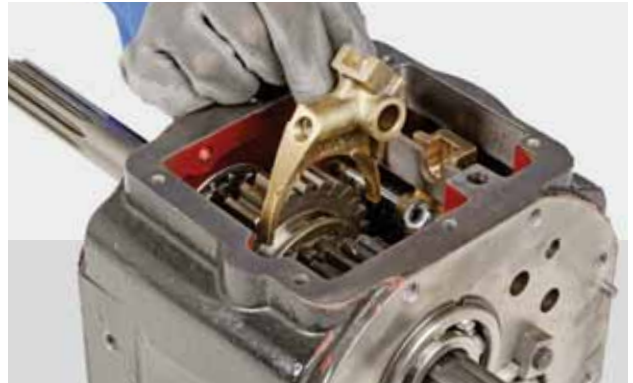
FIGURE 34: Note the position of the fork and remove.
