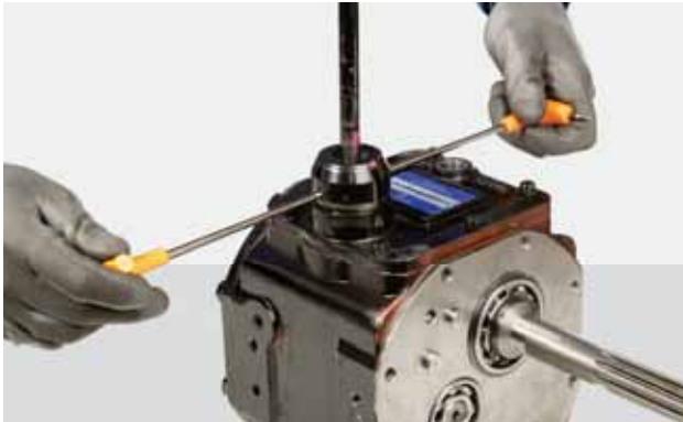
FIGURE 107: Adjust the lever adjustment pins and reset the gap to zero.
