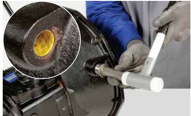
FIGURE 116: Only if removed, use a driver to install the bushing in its seat.
