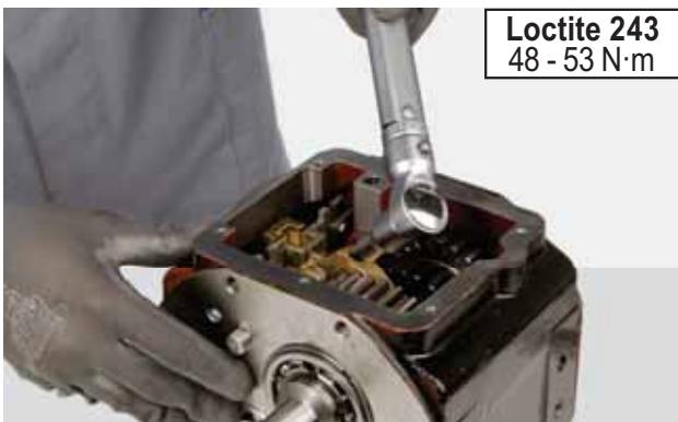
FIGURE 95: Install the fork lock nut and tighten to 48 - 53 N·m.
