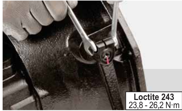
FIGURE 121: Install the lever and block with screw, and tighten to 23.8 - 26.2 N·m. Refer and keep to the positions marked during disassembly.
