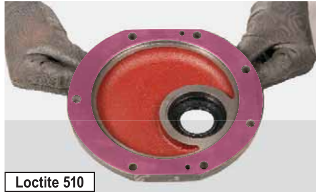
FIGURE 97: Apply LOCTITE 510 to the machined surfaces.
