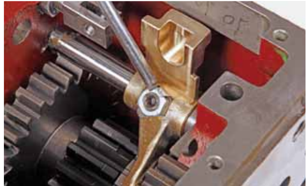
FIGURE 79: Bend the position stop. Do not overlap the folded material.
