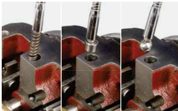
FIGURE 24: Using a magnet remove spring, spacer, and ball.
