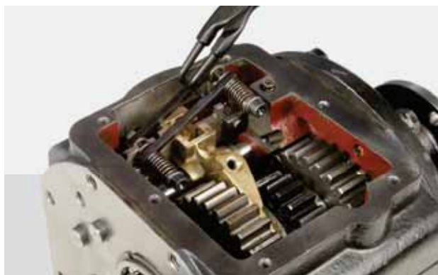
FIGURE 23: Remove the gear selector yoke.
