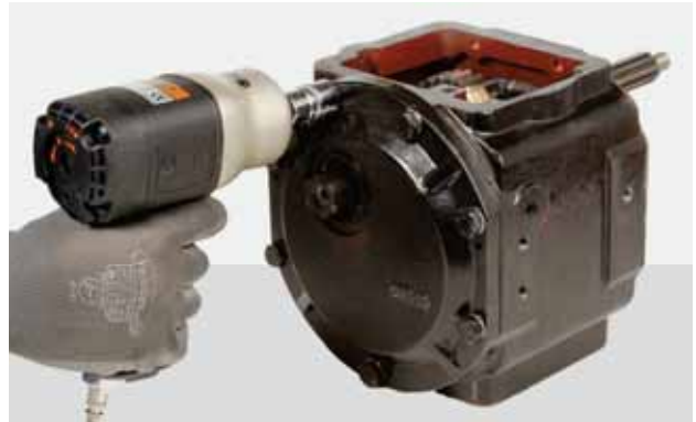
FIGURE 28: Loosen and remove the cover screws and washers.
