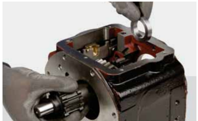
FIGURE 86: Fit the spacer onto the input shaft.
