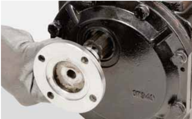
FIGURE 100: Install the flange onto the output shaft.
