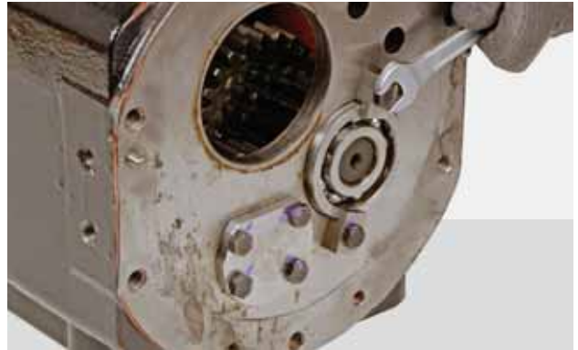
FIGURE 52: Remove screws and mechanical endstops.
