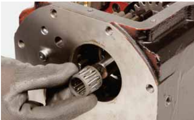
FIGURE 90: Lubricate and install the roller bearing.
