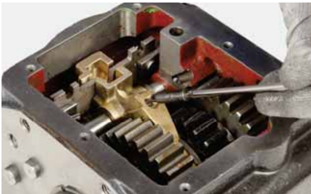
FIGURE 32: Remove the yoke capscrew.
