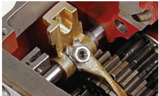
FIGURE 48: Remove the caulk from the position stop.
