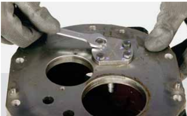
FIGURE 62: Remove the idler gear support capscrews.
