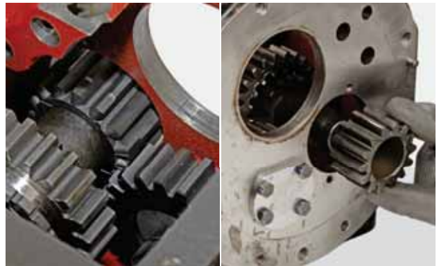
FIGURE 54: Remove the reverse gear as shown above.
