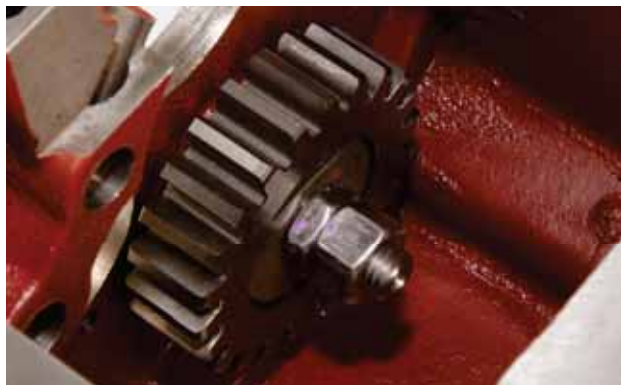
FIGURE 58: Loosen and remove the counternut and lock nut.
