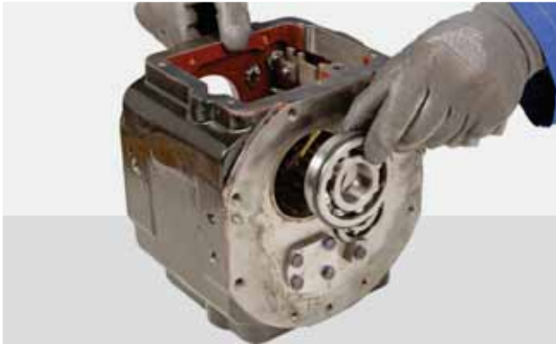
FIGURE 43: Remove the bearing.
