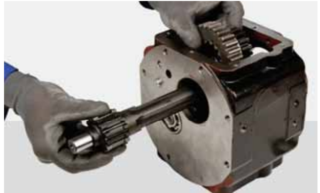
FIGURE 85: Insert the input shaft in position.
