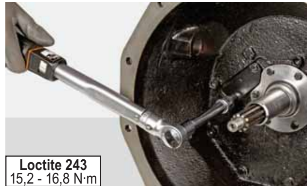
FIGURE 115: Coat the screw threads with Loctite 243 and tighten to a torque of 15,2 - 16,8 N·m.
