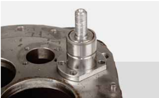
FIGURE 63: Replace the complete support if the thrust block is damaged.
