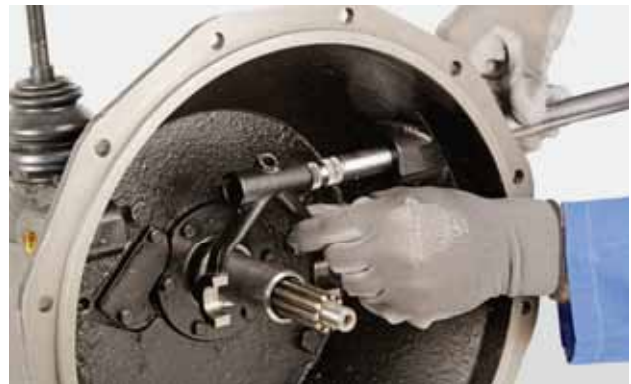
FIGURE 117: Assemble the pin and pressure plate yoke as previously marked.
