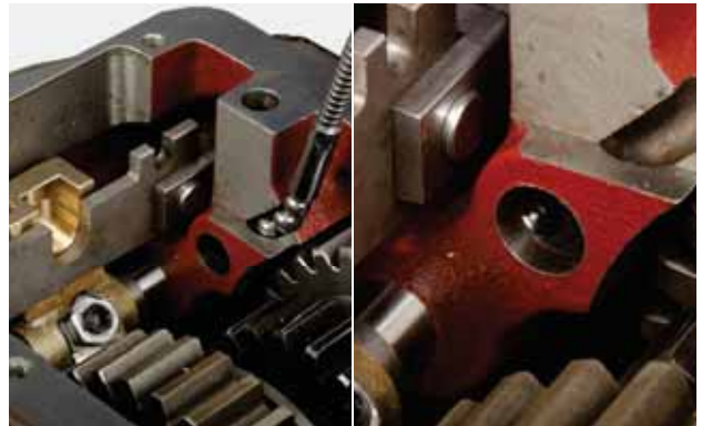
FIGURE 92: Install the three gear detent balls.
