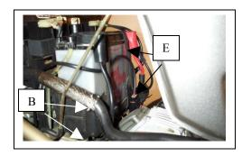
**STEP #3**—Install the fuse in the fuse-holder. Attach the wires to the socket. The center terminal is plus and the outer ring is negative (see dwg below). Apply either dielectric grease or Vaseline to the terminals. Use a voltmeter to check if the polarity is correct.
