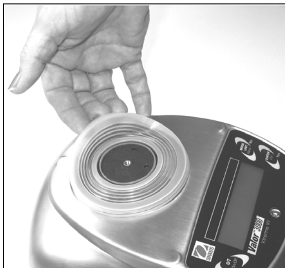
Figure 3-1. Proper way to lift off Seal.
