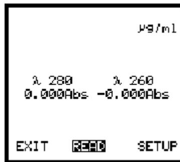
Remove the sample blank from the chamber and insert the unknown sample. Close the sample chamber lid. Select **READ** and the instrument will measure at both points (even when only 280nm is required):
