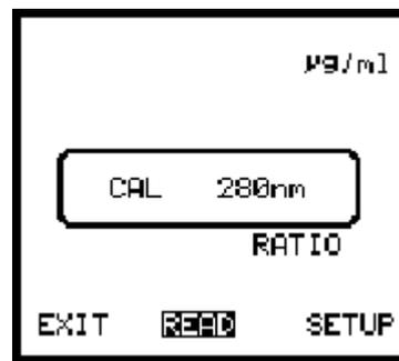
If the reference wavelength option is selected a third calibration will be performed at the nominal reference wavelength of 320nm. All 3 values will be shown on the instrument display.
