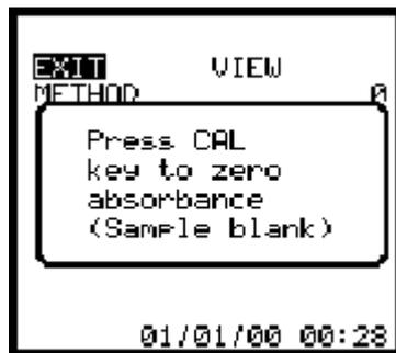
Press the **CAL** key again with a sample blank present in the sample chamber. The display will momentarily show **CAL**.
