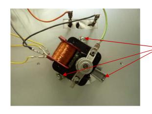
DISCONNECT WIRING FROM FAN
