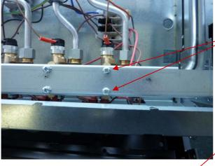
PULL FORWARD INNER FACIA PANEL TO GAIN ACCESS TO THE 2 X TAP SECURING SCREWS
