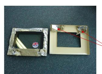
WITH THE SECURING SCREWS REMOVED THE INNER PANEL CAN NOW BE SEPARATED FROM THE OUTER PANEL
