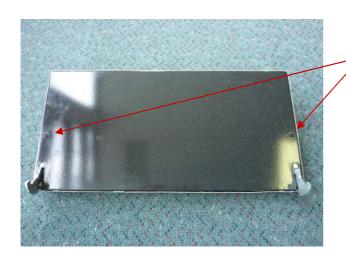
REMOVE 2 X SCREWS ON THE INNER DOOR PANEL AND 2 SCREWS AT THE BOTTOM OF THE PANEL TO REMOVE THE HINGE FRON THE INNER DOOR PANEL
