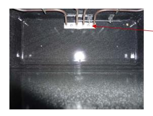
REMOVE THE 2 SCREWS SECURING THE ELEMENT BRACKET TO THE CAVITY AND PULL THE ELEMENT FORWARD TO REMOVE
