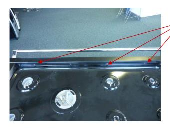
REMOVE 6 X SCREWS AT THE REAR OF THE FACIA PANEL AS SHOWN
