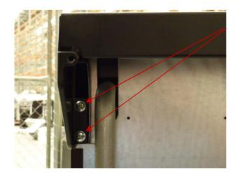
REMOVE 4 X SCREWS (2 EITHER SIDE) AS SHOWN THAT SECURES THE VENT TRIM
