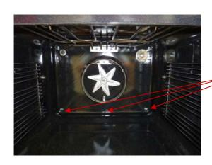
FOLLOW STEP 6 AND REMOVE THE REAR SERVICE PANEL REMOVE REAR FAN COVER REMOVE 3X SECURING SCREWS FROM INSIDE THE CAVITY
