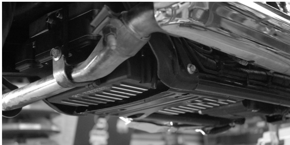
BAKER 1.5 OIL PAN INSTALLED, FIGURE 11
