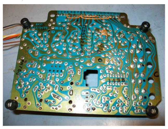
If you are using the exciter TLD513x observe note 409 on the schematic of manual # 68P81008E40-L. It says to bypass R431 (33 ohm) for 1-4 frequency operation. It's located on the input of IC401, pin 14. Other radio versions don't have this. And some (compa) types don't use the IC401 either.
