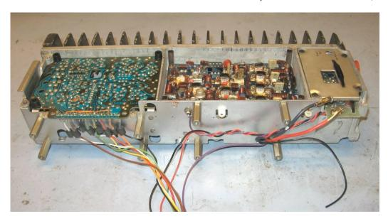
Now, you can install the exciter board in the chassis as show here. Then do the wiring for the power control board-3 wires, ground, A+ and control voltage. The latter connects to the PA control transistor. In this view a feed-though cap was used however, OEM just has the wire go through a hole in the chassis. Above view is the top of the chassis.
