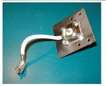
The (old) OEM coax with a RCA connector at one end was used to plug into the power control board. The other end was cut off and prepped for soldering directly onto the new N connector. Shown here is the completed subassembly (back and front) ready for the radio.
