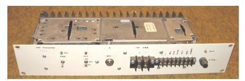
Serial 2 changed to the white panel standard. Shown here is the front of a finished transmitter. Notice there's a switch function to "lock on" the PTT line for transmitter testing under load. It was decided a ON-Center OFF-ON switch is sometimes awkward to use; disable being in the "center" position; one may run the switch to the down position and keep the PTT on, so this was changed to a ON-ON switch as shown here.
