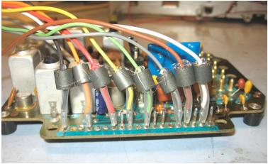
Here's the modified exciter board to the extent wires are soldered to the P904 (I/O) pins with heat shrink to increase reliability. Some of the unused pins are removed to assist the ferrite bead clearance (some others are left). The beads can reduce RFI on the lines if the site is (RF) hostile. A drop of glue will keep them in place. The unused pins that were removed are 2,3,5,6,10 and 14.
