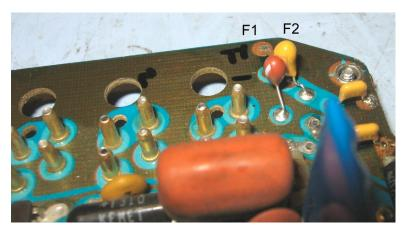
As of 2014 it's capable of 2-frequency operation. The F1 and F2 enable wires run out to TB1 for external control. In the picture above notice the "enable" lug-jumper on TB-1 terminals 7 and 8 for normal F1 operation. Terminal 10 is the fan control (discussed later).
