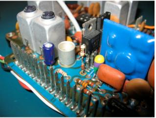
In the event the components needed replacement is an easy task working with the pins as solder mounts. In the right picture notice the blue capacitor next to Q406. If its larger in size move it slightly inward (angled leads) so it clears the chassis (rail) when installed.
