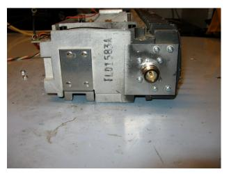
Without any of the front panel being built, this may be a good time to run the transmitter though its paces to look for any problems overlooked. In an extreme (bad) case you could stop here and start building a new one. Just clip the needed wires for power/control and put a load on the RF port, etc.
