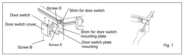
2. It confirms that an indicator lamp, the door switch and those wirings are being done, and the door switch ass'y is fixed on the door switch mounting plate with three screws B (M4 x 10 stainless steel (coating head)).(Fig. 2)
