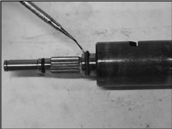
19. Install the shift drum into the case.
