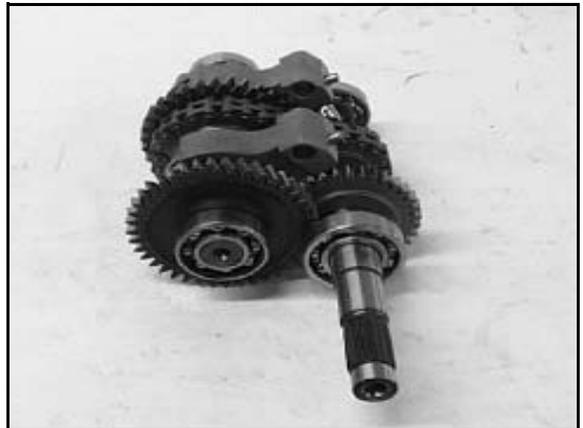
**NOTE: Installing the shift rail will aid in keeping the shift forks, shift dogs, and the springs in place.**
