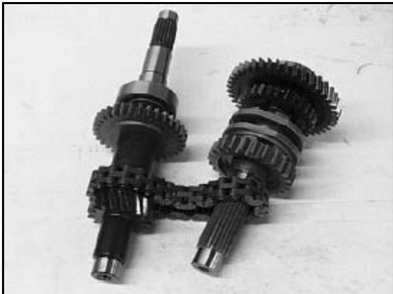
12. Install a new needle bearing, the low gear, the thrust washer and the snap ring. Use of a new snap ring is recommended.
