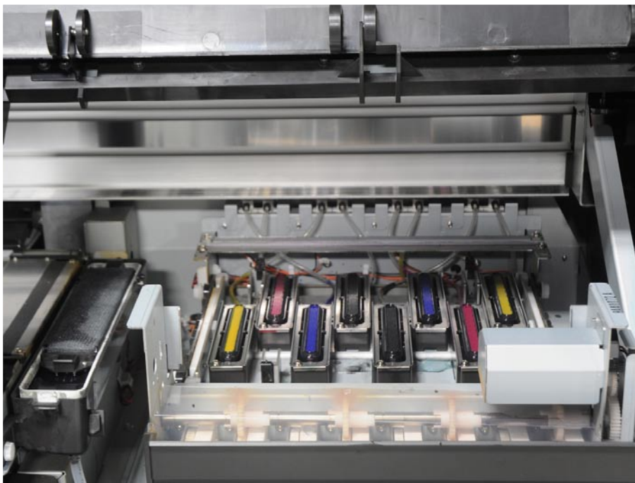
At the right side is located the capping station, that has the capping area, which prevents the nozzle of the printheads from drying.
