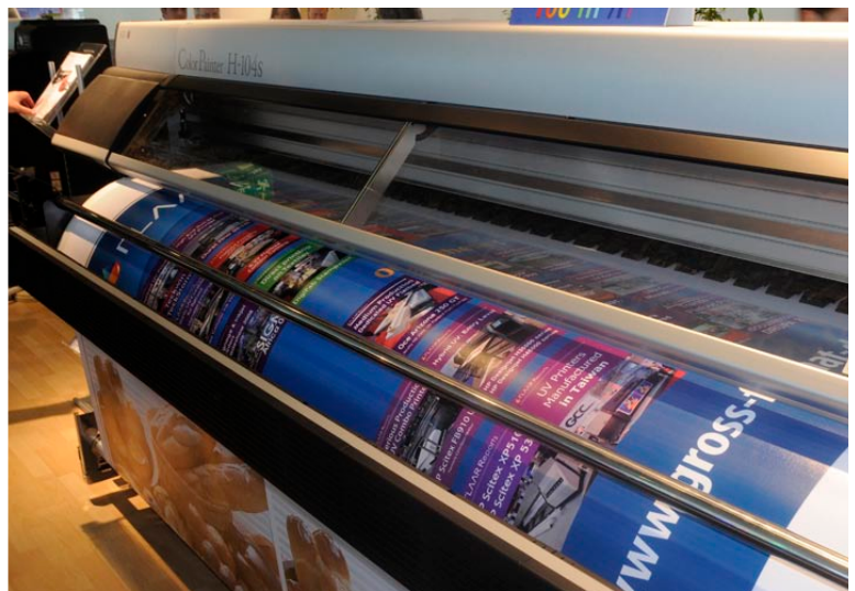
Banner being printed with a ColorPainter H-104 at VisCom Germany 2008.
