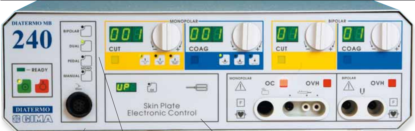
30690 CONTEMPORARY DUAL MODE MB 240 and 380 can be used in the same time in monopolar mode (by handle) and bipolar mode (by footswitch) A special electronic circuit (Skin Plate Electronic Control) continuously warns the plate to patient contact safety and unwanted short circuit in the connecting cable
