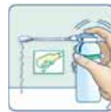
CHARGE custom applicator press valve until droplets start to form.
