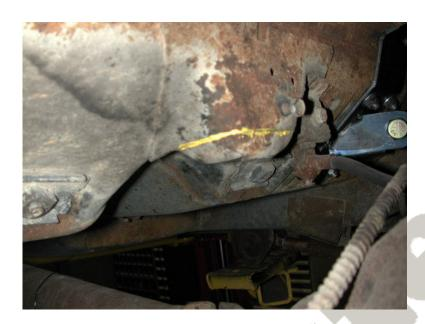
1. The pinion snubber mount must be cut on the line shown in the picture. This allows more clearance of the pinion for maximum drop.
