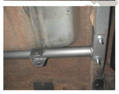
7. Lower the axle enough to slide the upper crossmember into place. The frame is wider towards the rear of the car as is the crossmember. Push it forward until it is tight between the frame rails, but make sure it is square. Drill two holes with a 7/16" drill bit.
