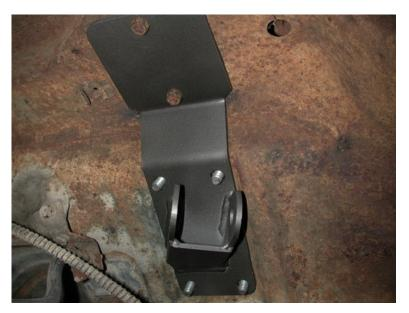
4. The upper bar mount will bolt to the bottom of the car using the factory shock bolts and locates off the factory shock mount.
