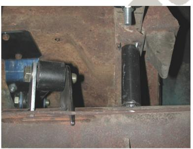
8. Remove the crossmember and drop the 3/8" U-bolt through the holes. Reinstall crossmember and tighten with 3/8" nylocs and flat washers.
