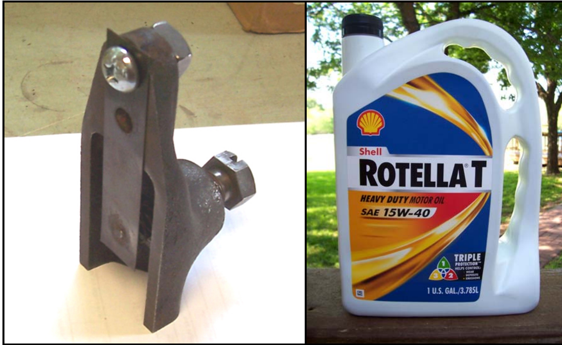
Figure 14-3 (A&B). John Deere “H” Oil Pressure Regulator Unit (left), and on the right is the “Author’s Choice” of oil for Two-Cylinders Tractors
