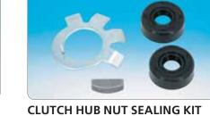
Convenient kit made by James Gaskets. Can be used with any 4-speed clutch as used in 1941 thru 1984, except those equipped with a diaphragm style clutch. Kit contains two double lip oil seals, a clutch hub key, and clutch hub lock plate.
