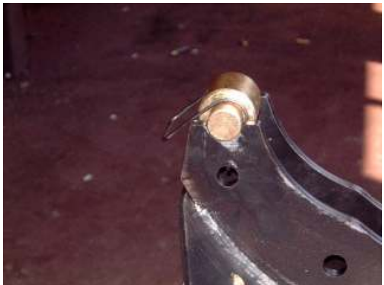
Fit the other retainer in similar manner in opposite direction.
