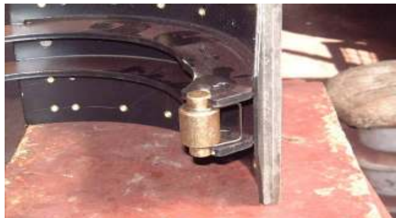
Finished position of Roller retainer. Fit Spring return spring onto brake shoe.
