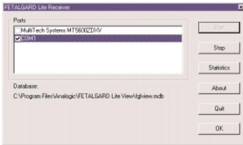
To enable or disable a port, the user must select the port by clicking its description in the list box. Then, if a port is disabled, it can be enabled with the "Start" button. If a port is enabled, it can be disabled with the "Stop" button. Enabled ports are indicated by a check mark next to the port description. Only one of the "Start" and "Stop" buttons will be enabled at any time.
