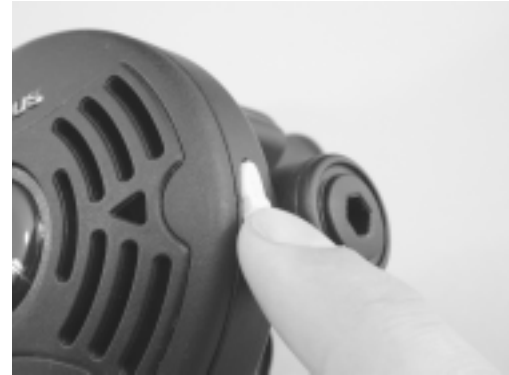
Figure 32. Press locking tab into place to secure front cover
