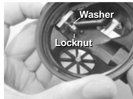
Figure 23. Install washer followed by locknut
