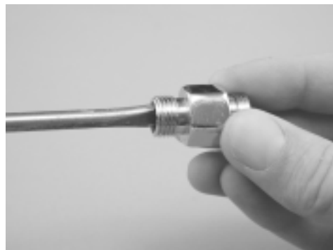
Figure 6. Unscrew adjustable orifice to disengage threads
