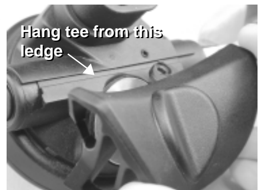
Figure 33. Hang exhaust tee on top edge of flange
