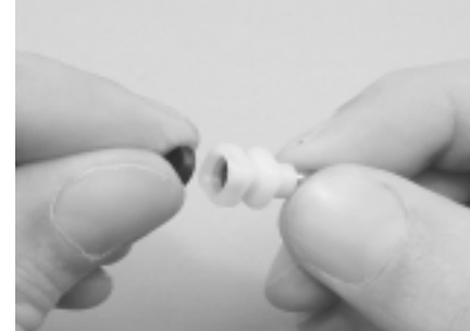
Figure 21. Press new LP seat into seat retainer
