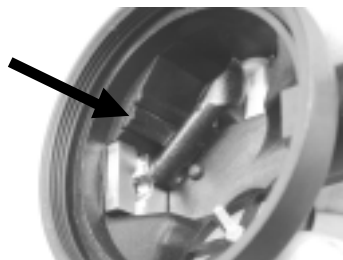
Figure 19. Venturi channel installed
