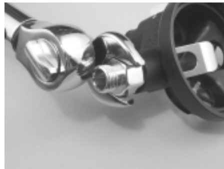
Figure 27. Torque inlet fitting to 60 inch-pounds
