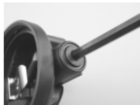
Figure 28. Install port plug
