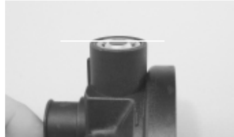
Figure 25. Tighten locknut until poppet is flush with valve body opening
