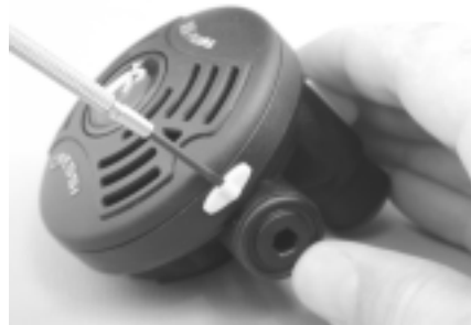
Figure 4. Removing the front cover locking tab (XS series only)
