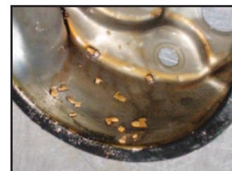
Contaminated Power Steering Pump Housing
