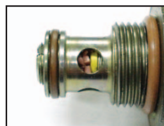
Blocked Modulating Valve
