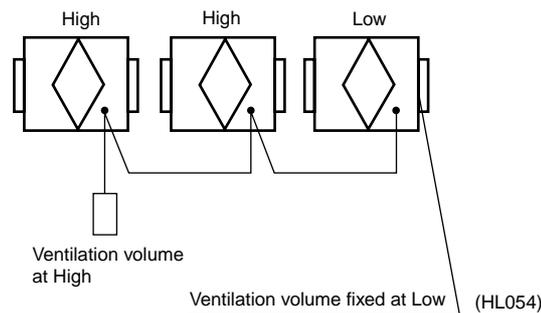
This setting method can be used when a group control system is connected with units having a different airflow capacity from other units in the system.
