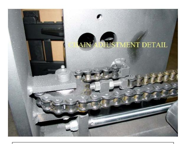
THE CHAIN TENSION ADJUSTMENT IS PROVIDED BY AN ADJUSTABLE CHAIN ANCHOR ON ONE END OF THE CHAIN LOCATED ON THE BACKSIDE OF THE BOOM. LOOSEN THE TWO LOCKING NUTS AND TURN THE ¾" NUT CLOCKWISE, LOOKING FROM THE END OF THE CHAIN ANCHOR, TO INCREASE THE CHAIN TENSION OR COUNTER CLOCKWISE TO REDUCE THE CHAIN TENSION.
