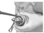
Attach the crank shaft onto the crankcase, and fix dowel pins into the crankcase.
