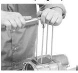
Fit a kit's cam chain in the crank shaft, and install the tensioner roller.
