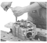
Being careful of the direction of the gear shift drum washer, tighten it to the specified torque with a hex bolt, and attach a rubber plug.
