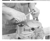
After applying Alumi Special a little to the threaded part of the stud bolts, attach stud bolts to the crankcase, and tighten them to the specified torque. Fix the stud bolt B, the shorter stud bolt, to the clutch side.
