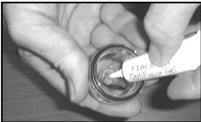
6. Fill reservoir with gel.
