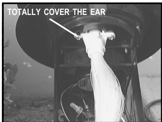
12. Secure "ears" under the screws.
