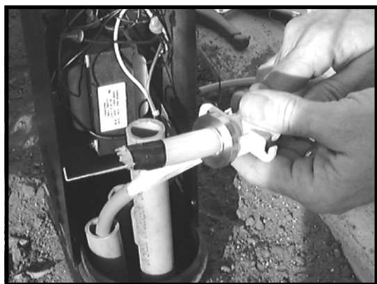
8. Screw on the cutting shield.
