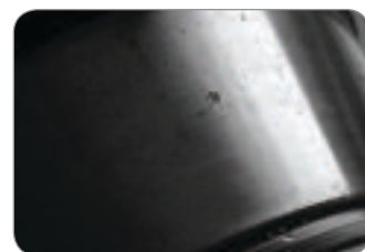
Surface appearance caused by electrical arcing during welding.
