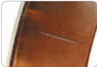
Dent across the race indicates a sharp high impact.
