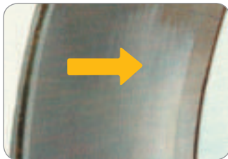
Severe sliding wear due to presence of hard abrasives.
