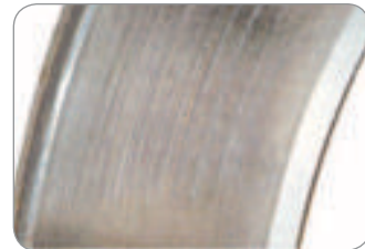
Heavy grooving by large hard particles in the lubricant.
