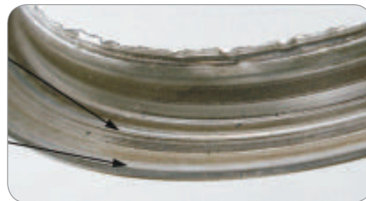
Axial Dirt Lip Pattern Bumper Lip Wear Pattern
