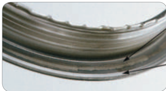
Axial Dirt Lip Pattern Bumper Lip Wear Pattern
