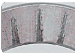
Typical surface appearance with repeated effects of vibration (called "false brinelling").
