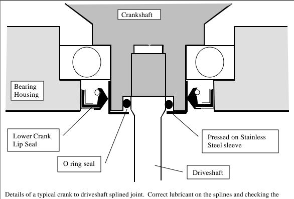
condition of seals should be part of every service where the gearcase is removed.
