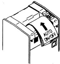
To shred a piece of paper too small to break the light barrier, press the FORWARD button (7) once to override the auto ON/OFF function. The shredder will continue to run until the FORWARD button is pressed again.
