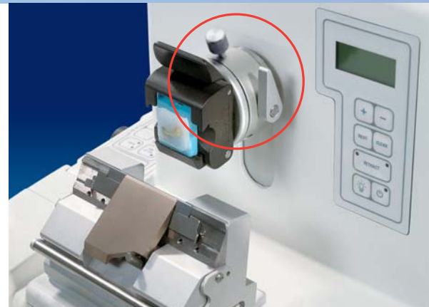
3. Press AUTO to make the specimen head rewind 5 mm.
