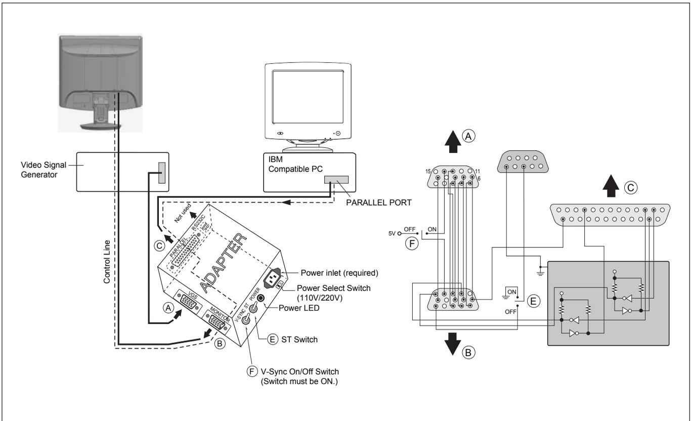
Figure 1. Cable Connection
