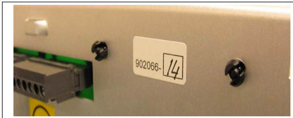
Figure 2-10A: DSS subassembly and tab number location
