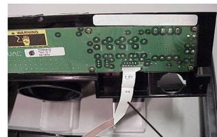
The top of the ribbon is marked with the word "UP" to aid in proper connection.
