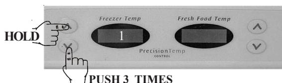
The freezer display will show “1”. The fresh food display will be blank. Each press of the freezer temperature up (Warmer) or the freezer temperature DOWN (Colder) key will step you through the service menu tests, “1” through “7”. Each press of the fresh food temperature UP (Warmer) or fresh food temperature DOWN (Colder) key will step you through variables of each test.
