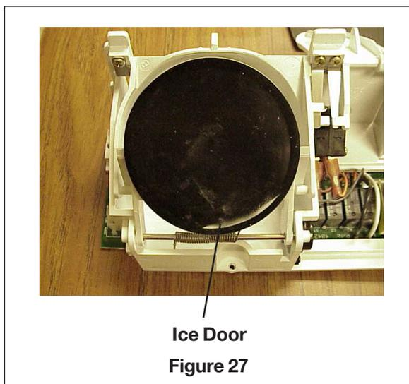
The ice door can be installed in the field with the internal chute heater to control moisture on the outside of the door. This may appear in certain areas with high humidity.
