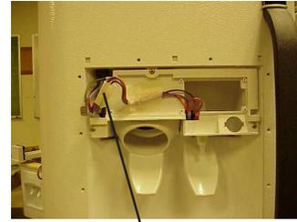
**Connector from door harness to actuator switches**
