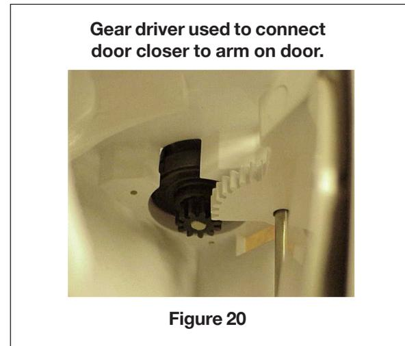
The closer can be replaced by removing 3 screws and lifting closer from housing. The door is held in place with a shaft at the top. The spring that holds the door closed and sealed against the housing is over the shaft and can be replaced by using a small punch and removing the shaft. (See Figure 21)
