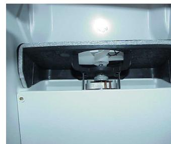
Evaporator Fan Motor Assembly
