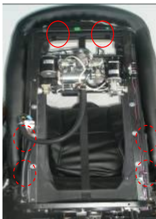
Screws fastening the front cover to the back frame (6 PCS)
