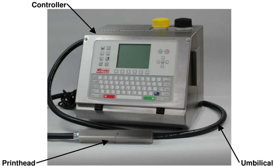
The keyboard and display are used to operate the system. The power switch is used to turn the system on and off. Ink and Makeup fluids are added at the top of the systems.
