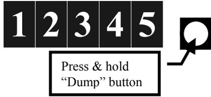
With the digital display the logic board is now able to convey exactly why the “Empty” LED is lit. Press the “Dump” button **while the “Empty” LED is lit**. On the Light-up display the meter count will go away while holding the button down. These are the error code definitions:
