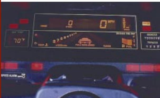
The POWER mode increases the upshift and downshift points. It is deactivated by the vehicle speed and the throttle angle, i.e., if the speed is equal to or greater than approximately 40 MPH with a light throttle, deactivation is immediate.
