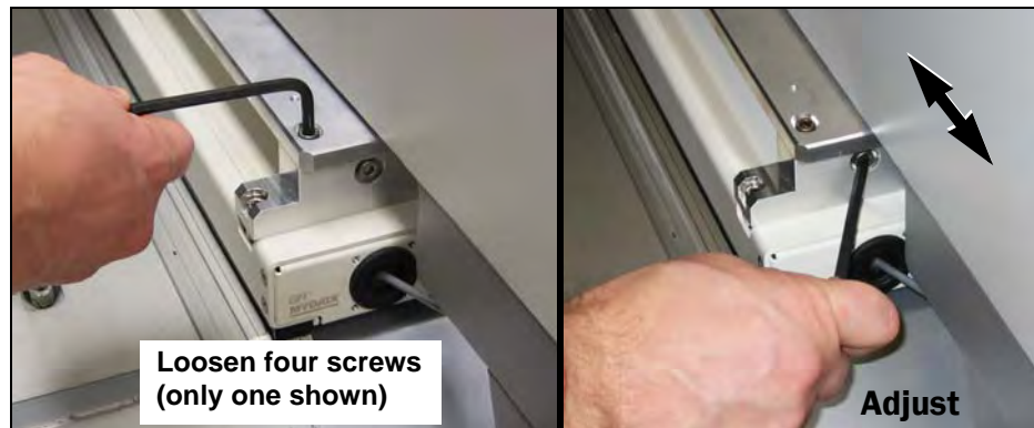
Figure 2-8—Adjusting the pick point.
