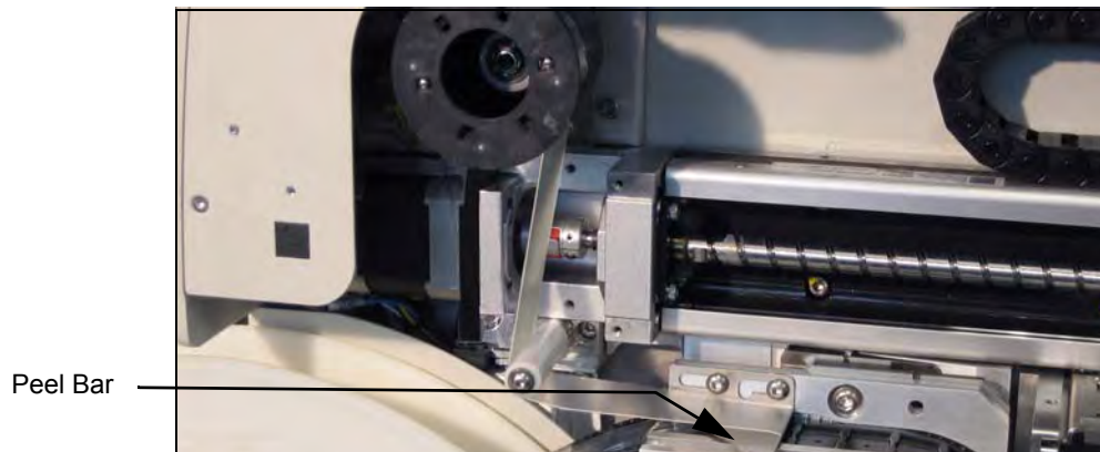
Figure 3-17—XLF Models ONLY: Loading device tape. Note that the reel winds up Cover Tape in the opposite direction than standard models.
