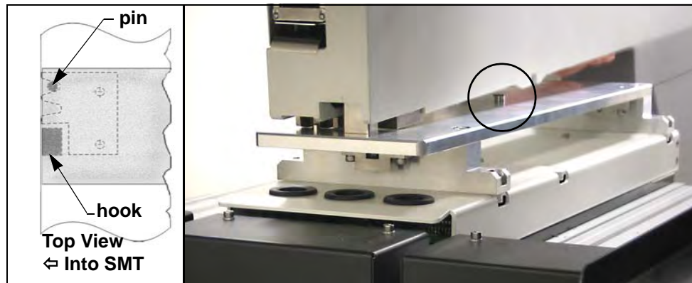
Figure 2-6—Installing RoadRunner onto the Feeder Bank Adapter. A dowel on the Adapter (circled) mates with the RoadRunner nose.
