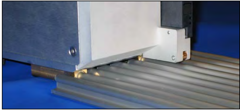
Figure 2-25—The SMT Adapter on SIPLACE X RoadRunner mates with ribs on the Feeder Bank.
