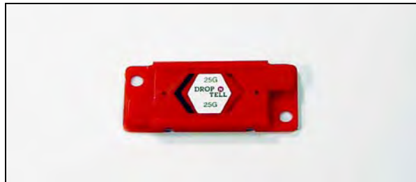
Figure 2-1—Shock Indicator is Indicating that an Impact has Occurred (Left Side, black arrow [<])
