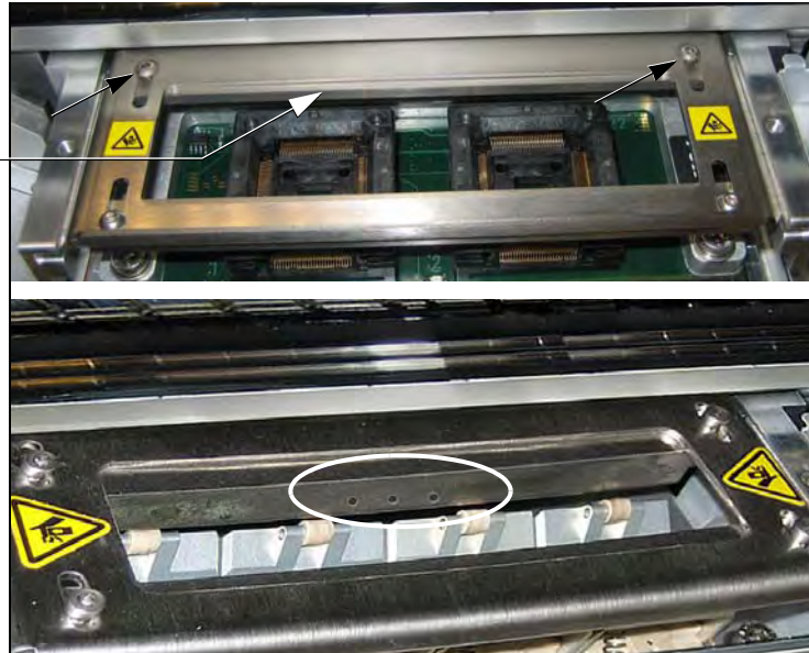
Figure 3-8—Adjustable Actuator Plates: Standard (top) and HIC, identifiable by the three dots.
