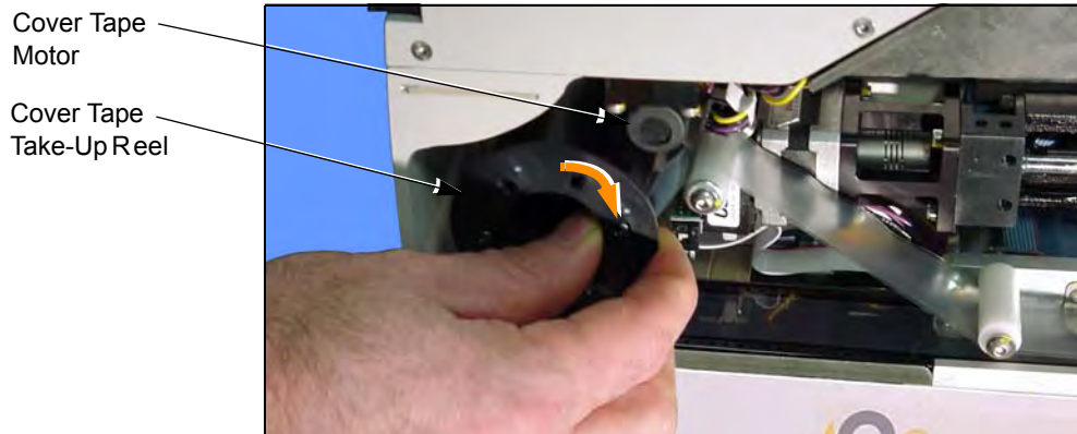
Figure 1-4—Loading Cover Tape [Siemens model shown]. Note that on XLF Models the cover tape rotation is in the opposite direction.
