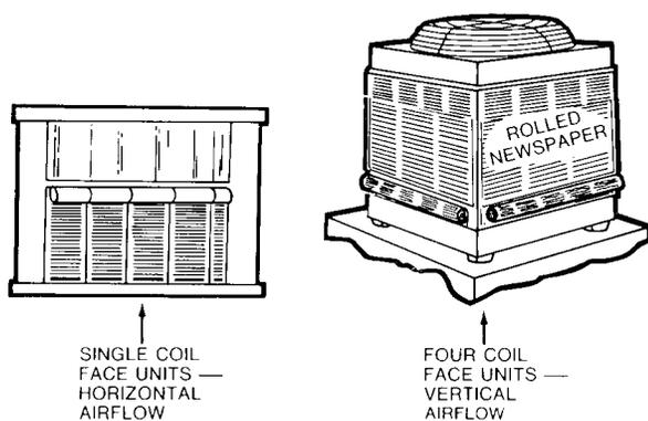
Coil Blockage For Dwyer Defrost Control Adjustment
