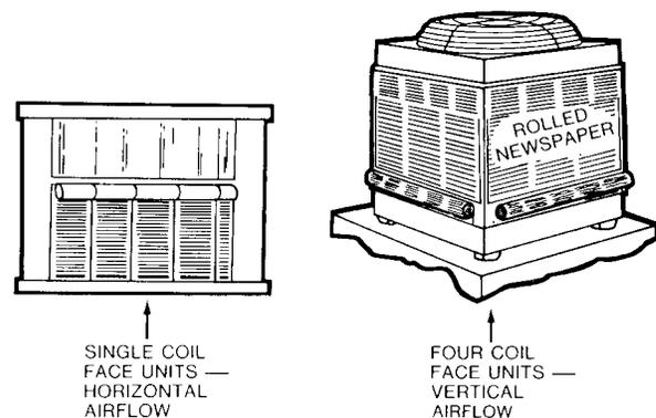
Outdoor Coil Blockage For Control Adjustment
