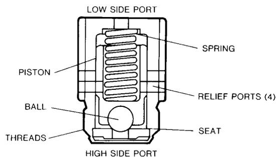
Compressor Internal Pressure Relief Valve
