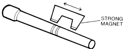
Testing Check Valve With A Magnet
