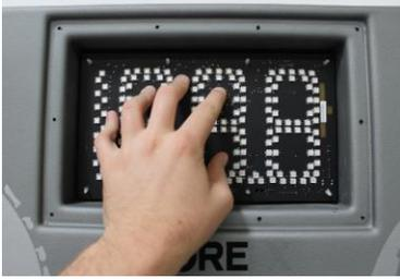
5. All 8 stand-offs need to clip in the hole. It is essential to go around each stand-off and test if the clip is set. Push up on each stand-off listening for a clipping noise that ensures the clips have set.
