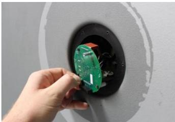
4. To disconnect the existing target board, remove all wire connectors (8-pin, 2-pin) on the back of the board. To remove the connectors hold on firmly to the 8-pin or 2-pin connector and “wobble” it until the connector becomes free (DO NOT pull by the wires). Start with the connector that has the shortest wire. Do not remove connectors by pulling on the cables. This may break one or more of the wires. Your old target board is now removed.
